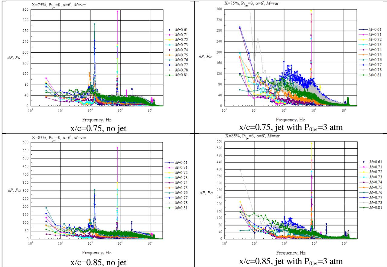
Figure 5: Spectra of pressure pulsations for  $\alpha=6^\circ$  for baseline (left) configuration and tangential jet blowing (right) with  $P_{\text{jet}}=3$  atm
