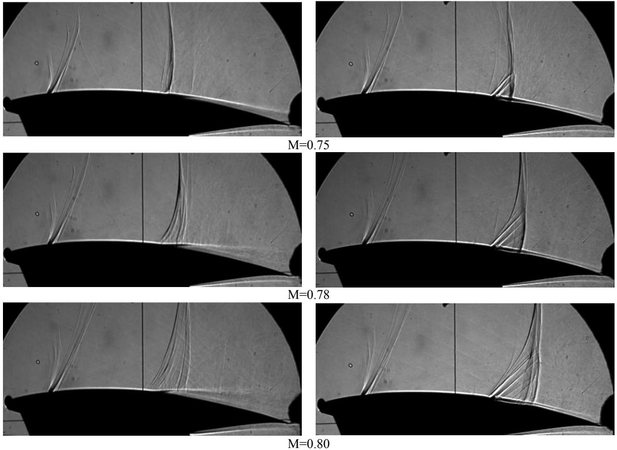
Figure 4: Shadow images for baseline configuration (left) and configuration with tangential jet blowing (right) at  $P_{0\text{jet}}=3 \text{ atm}$ ;  $\alpha=5^\circ$
