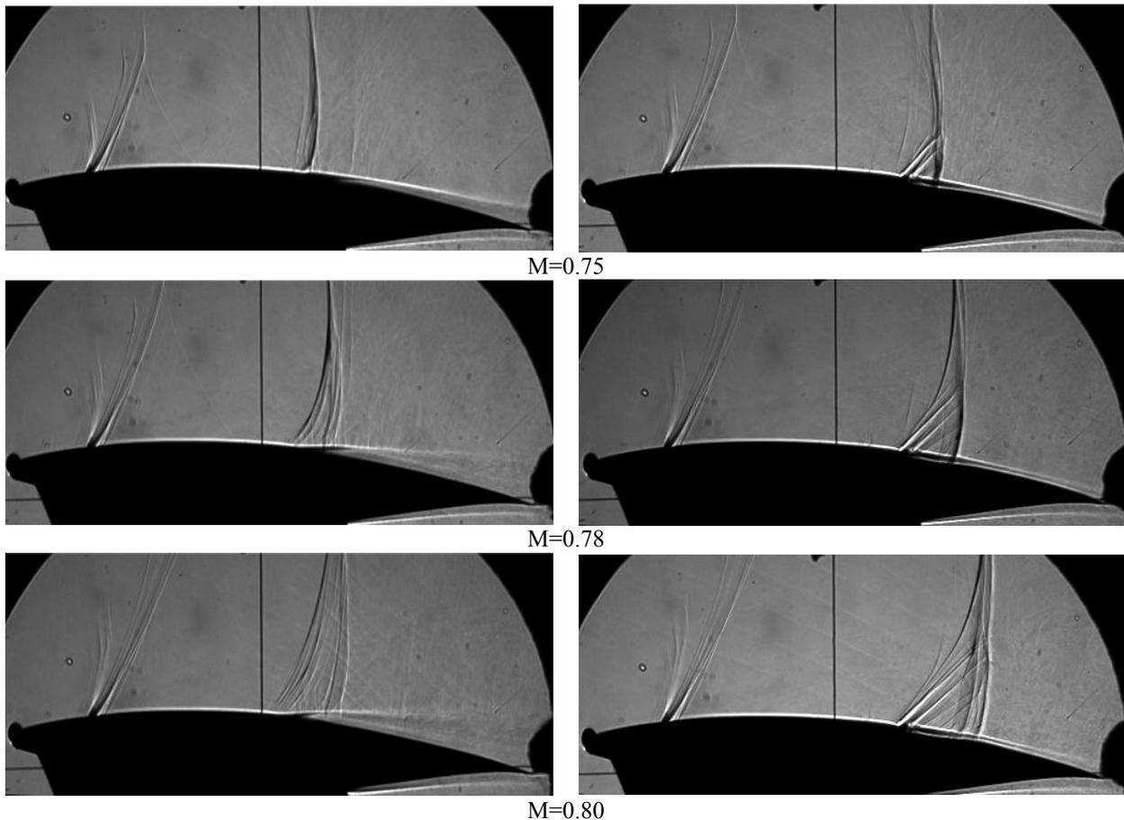
Figure 4: Shadow images for baseline configuration (left) and configuration with tangential jet blowing (right) at  $P_{0jet}=3$  atm;  $\alpha=5^\circ$
