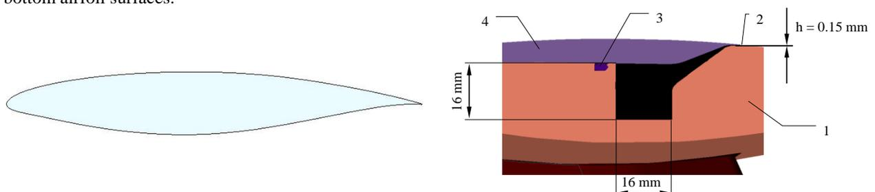
Figure 2: Airfoil P-184-15SR and slot nozzle cross-section; 1 – wing, 2 – slot nozzle, 3 – seal, 4 – cover of the air chamber
