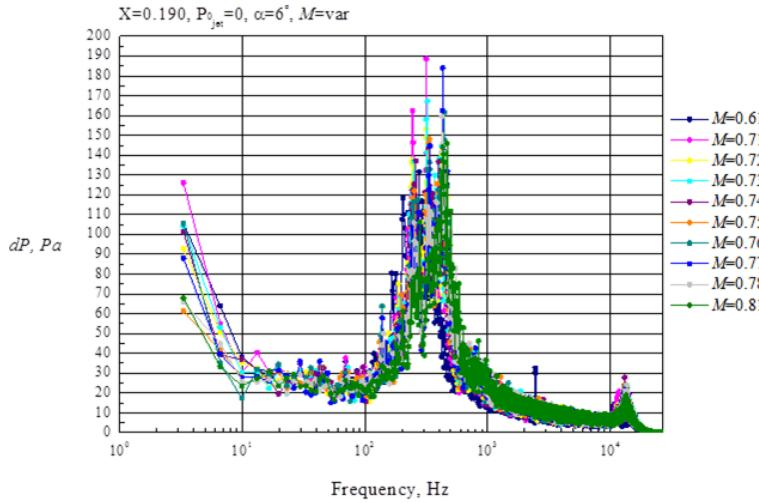
Figure 6: Spectra of pressure pulsations on the wall at  $x/c=0.190$  without jet blowing
