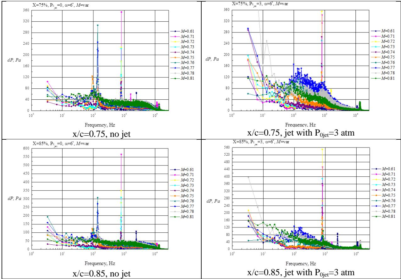
Figure 5: Spectra of pressure pulsations for  $\alpha=6^\circ$  for baseline (left) configuration and tangential jet blowing (right) with  $P_{0\text{jet}}=3 \text{ atm}$
