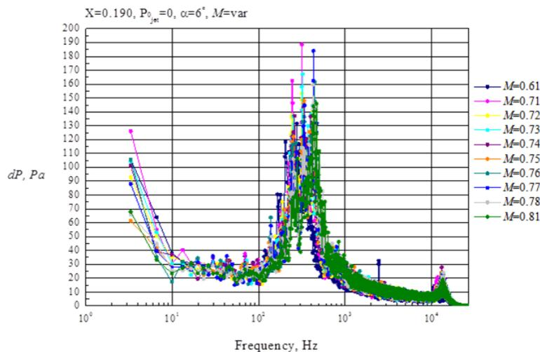
Figure 6: Spectra of pressure pulsations on the wall at  $x/c=0.190$  without jet blowing
