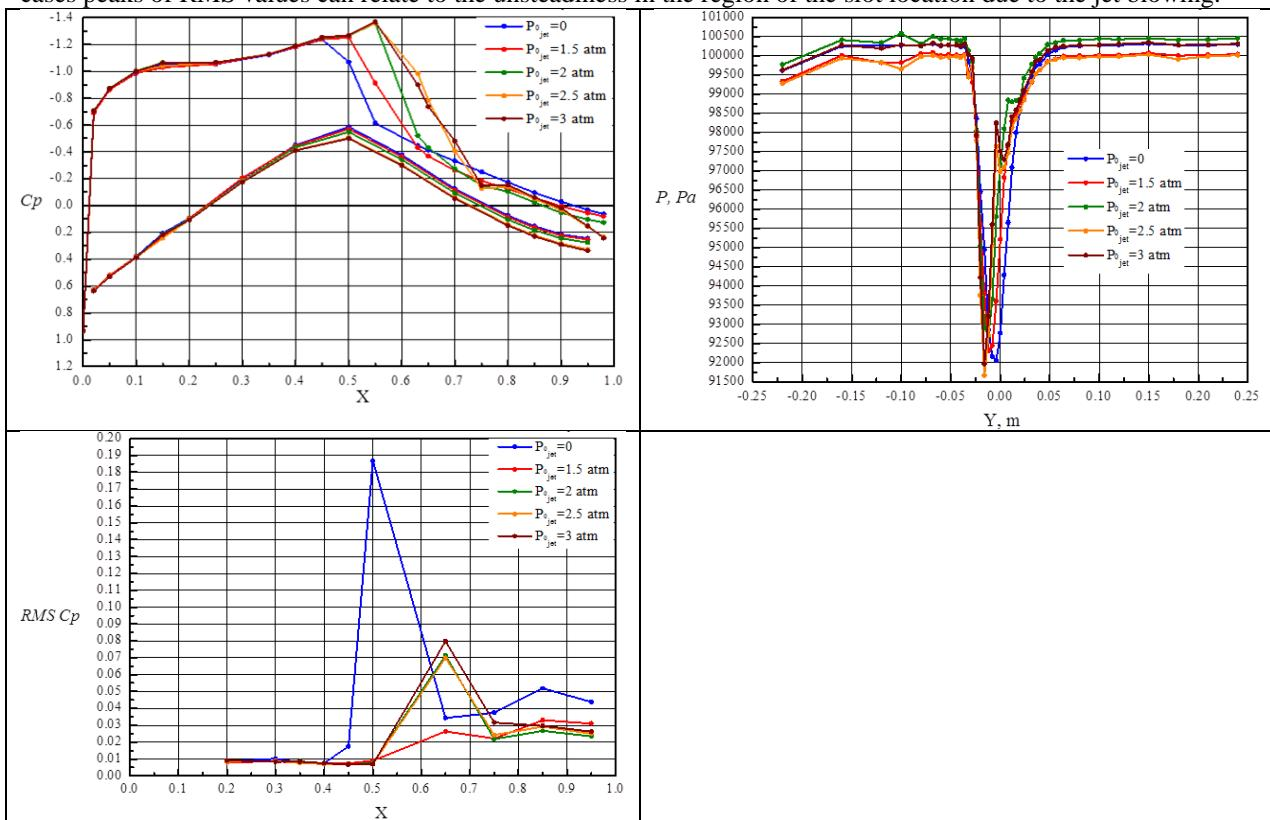
Figure 3: Pressure coefficient  $C_p$ , RMS  $C_p$  and total pressure in the wake downstream of the model for  $M=0.75$ ,  $\alpha=6^\circ$
