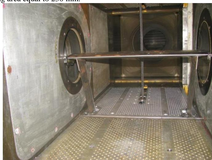
Figure 1: T-112 TsAGI transonic wind tunnel with the model, view from leading edge
