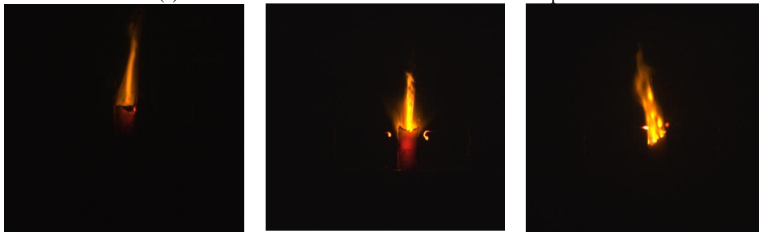
(1) 0.481MPa (2) 1.477MPa (3) 2.545MPa (b) Flame characteristic of KD-2 under different backpressure
