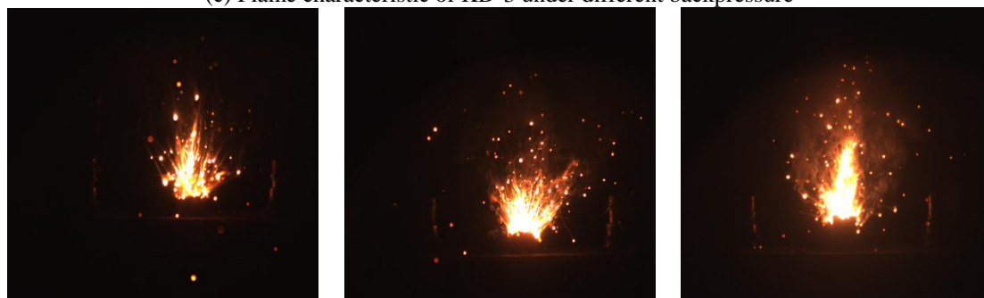
(1) 0.469MPa (2) 1.465MPa (3) 2.53MPa (d) Flame characteristic of KD-4 under different backpressure
