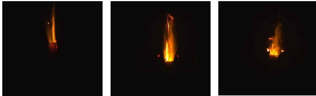
(1) 0.496MPa (2) 1.475MPa (3) 2.37MPa (a) Flame characteristic of KD-1 under different backpressure
