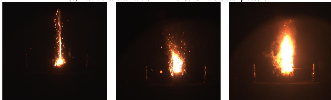
(1) 0.469MPa (2) 1.475MPa (3) 2.544MPa (c) Flame characteristic of KD-3 under different backpressure
