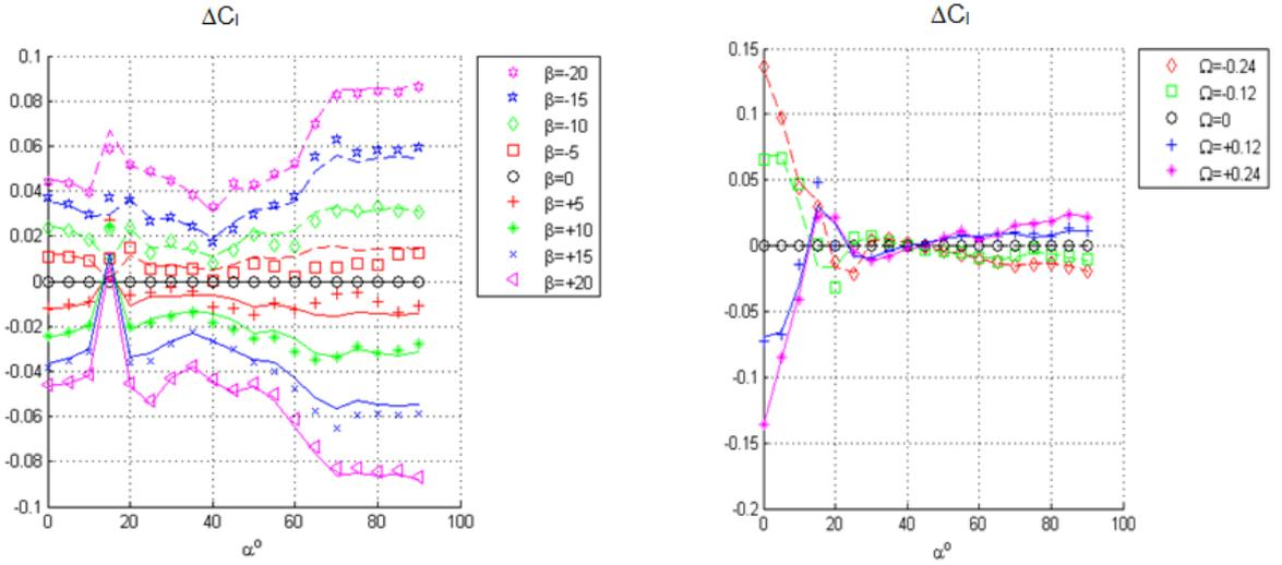
Figure 1: Roll moment dependence on sideslip angle and non-dimensional angular rate
