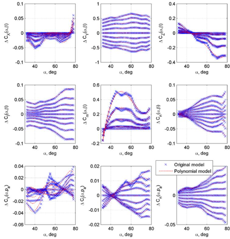
Figure 6: Look-up table data and polynomial fit for  $\Delta C_i(\alpha, \beta)$  and  $\Delta C_i(\alpha, p_a)$
