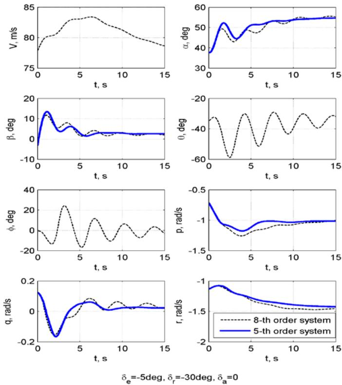
Figure 4: Comparison of trajectories near spin motion according to 8<sup>th</sup> order and 5<sup>th</sup> order equations
