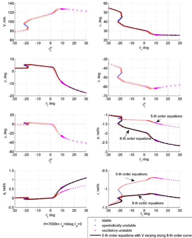
Figure 3: Equilibrium solutions for different rudder deflections.
