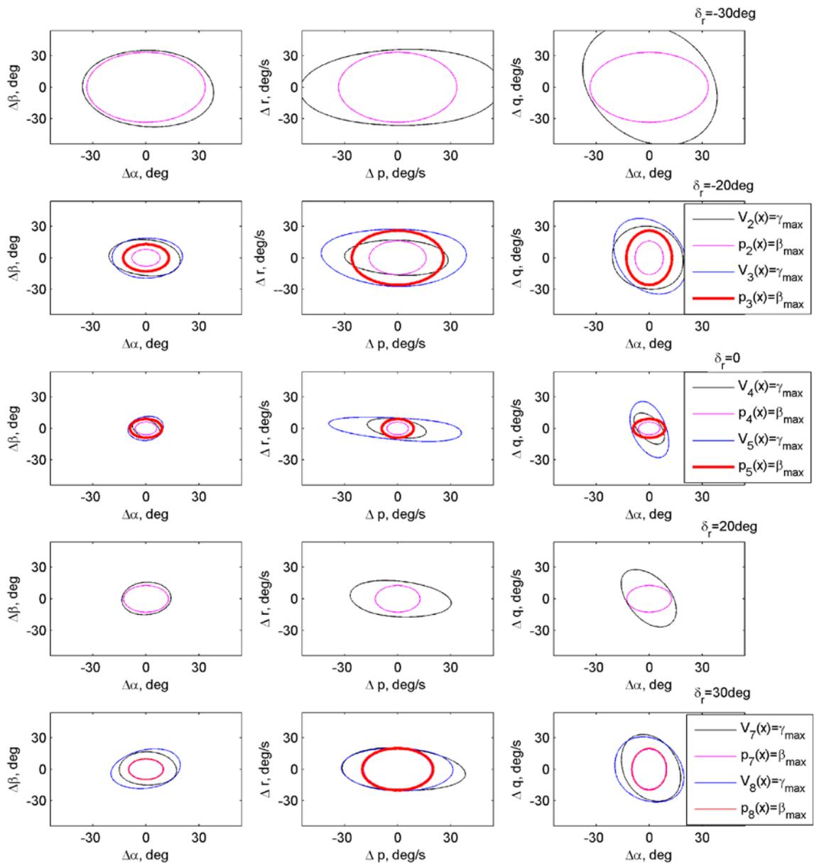
Figure 12: Projections of sublevel sets of Lyapunov functions and estimated ellipsoidal approximations for spin regimes from Table 1
