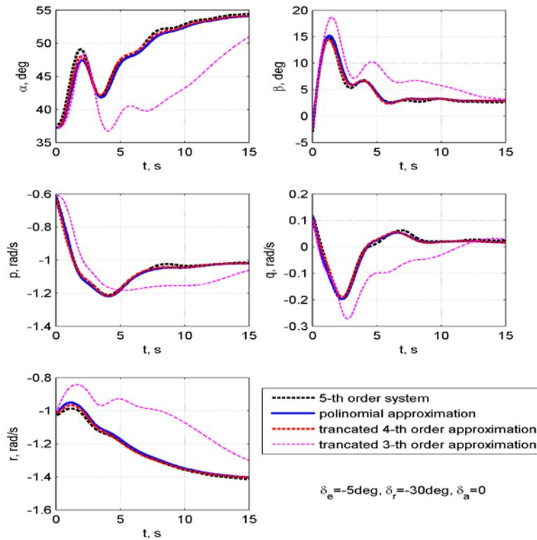
Figure 8: Comparison of time histories of motion parameters for 5th order equations and polynomial approximations
