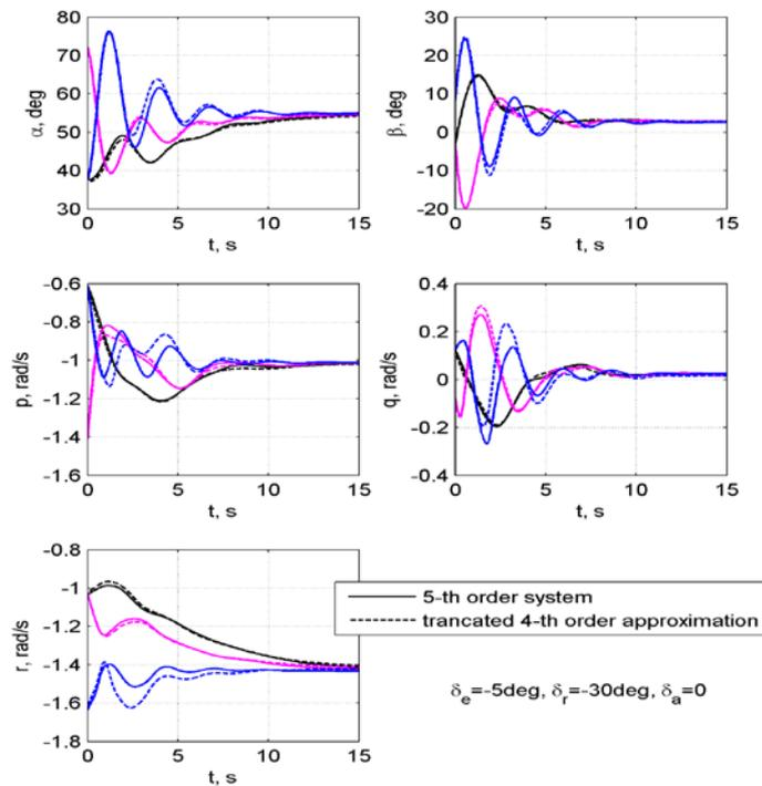
Figure 9: Comparison of time histories of motion parameters for the original 5th order equations and polynomial approximations for different initial conditions.
