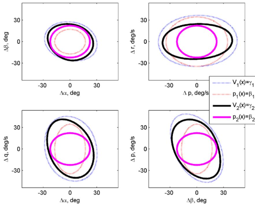
Figure 11: Projections of sublevel sets of Lyapunov functions and estimated ellipsoidal approximations for  $N=\text{diag}(5.25,5.25,1.31,1.31,1.31)$  ( $V_1, p_1$ ), and  $N=\text{diag}(1,1,1,1,1)$  ( $V_2, p_2$ ).
