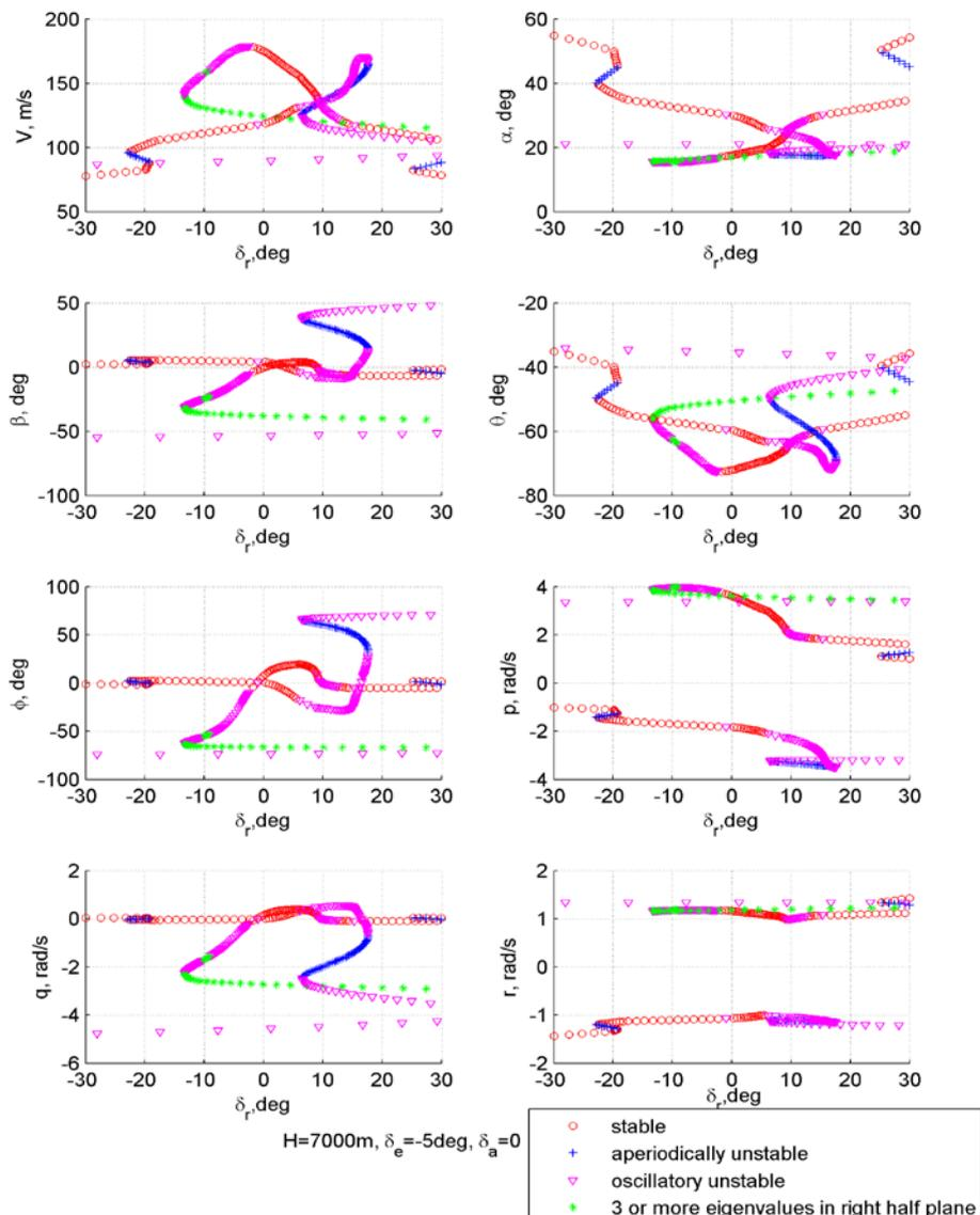
Figure 2: Equilibrium solutions for different rudder deflections,  $\delta_e = -5, \delta_a = 0$
