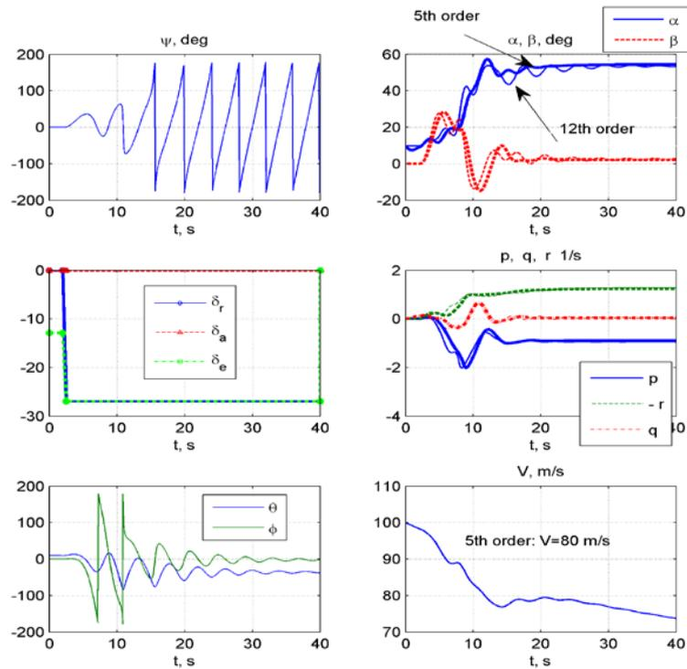
Figure 5: Entering into spin motion from a straight-and-level flight: 12<sup>th</sup> order and 5<sup>th</sup> order equations
