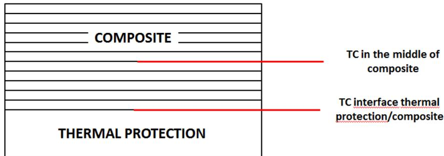
Figure 1 Scheme of TC positioning on composite/TP panel
