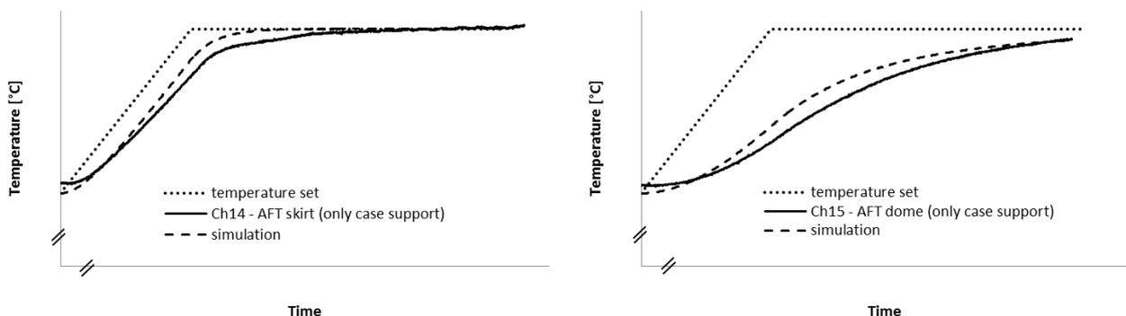
Figure 3 Temperature trend on AFT skirt and on AFT dome (only case support)
