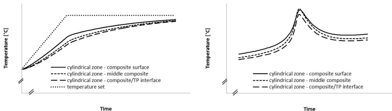
Figure 11 Temperature distribution of the composite material in the cylindrical zone
