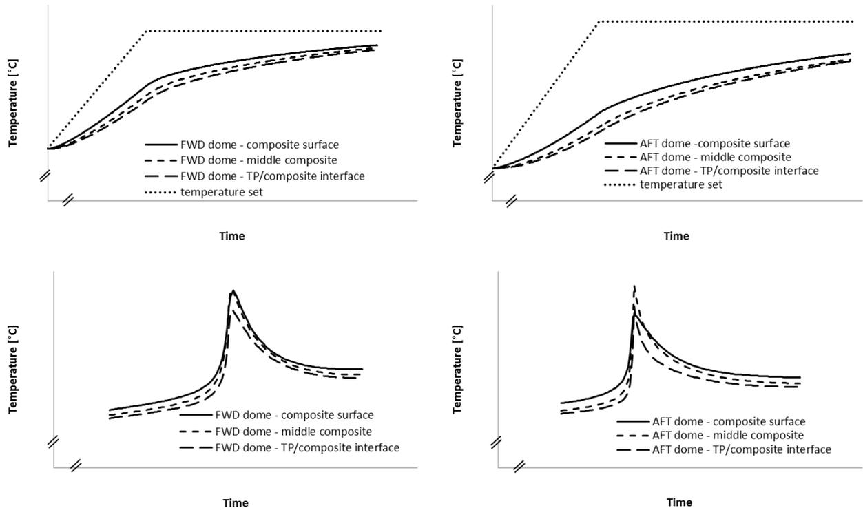
Figure 7 Temperature distribution for FWD and AFT dome in the composite material
