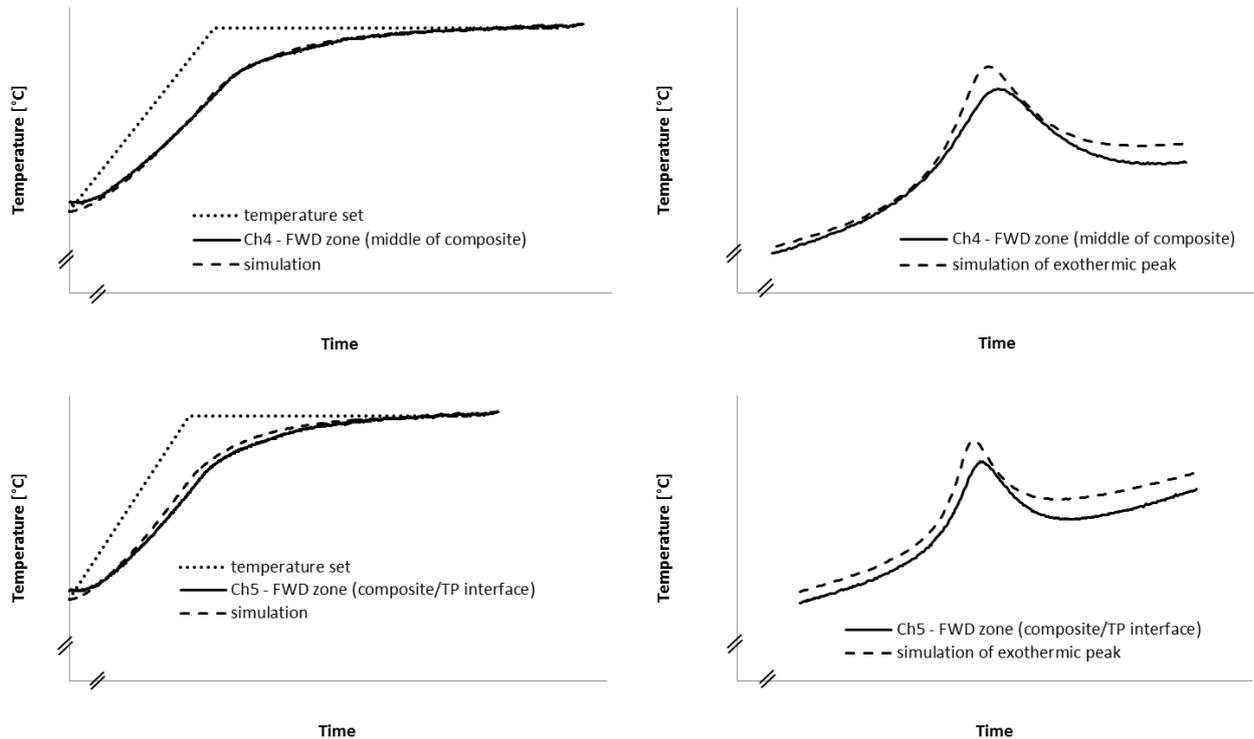
Figure 4 Temperature trends on FWD zone in composite material
