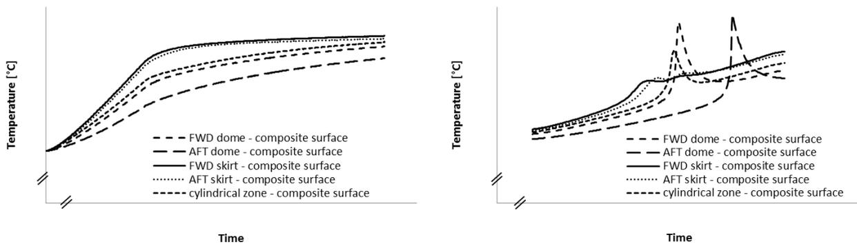
Figure 13 Temperature distribution of the composite material on the surface of SRM casing
