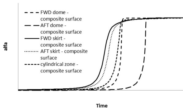
Figure 14 Conversion degree of the composite material on the surface of SRM casing
