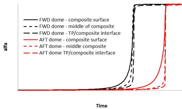
Figure 8 Conversion degree for FWD and AFT dome in the composite material
