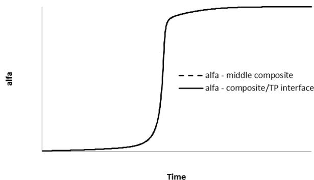
Figure 5 Degree of cure of the composite material panel
