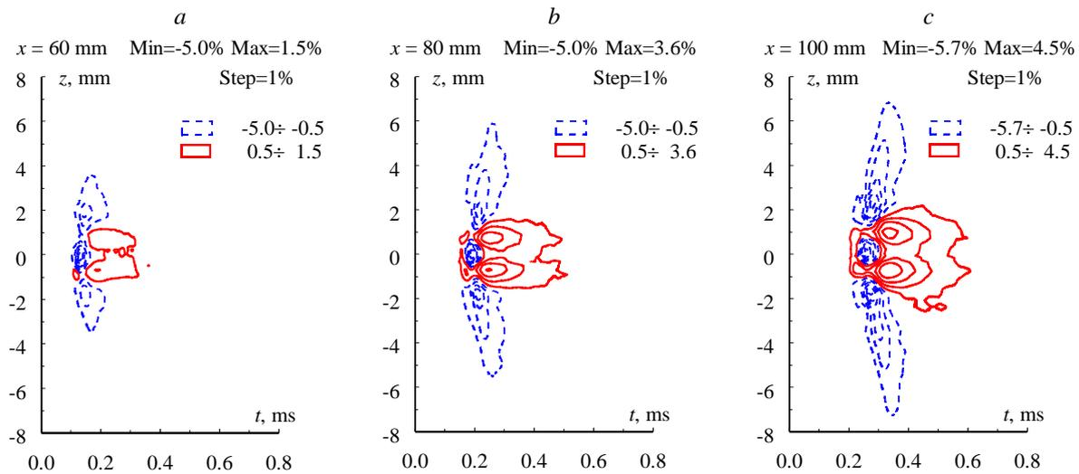
Figure 5: Contour lines of the mass-flow pulsations of the wave packet in the plane  $(z, t)$  at  $x=60$  (a),  $80$  (b) and  $100$  (c) mm.
