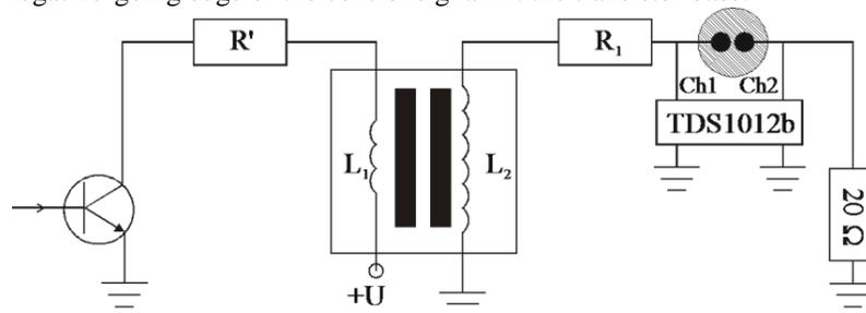
Figure 2: Discharge ignition schematic.
