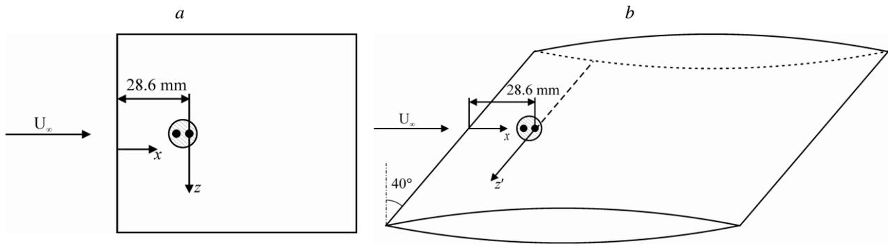
Figure 1: Experimental models. *a* – flat plate; *b* – swept wing.
