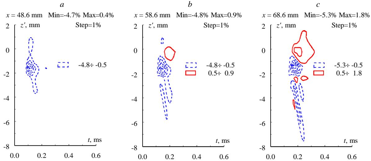
Figure 7: Contour lines of the mass-flow pulsations of the wave packet in the plane  $(z', t)$  at  $x=48.6$  (a),  $58.6$  (b) and  $68.6$  (c) mm.
