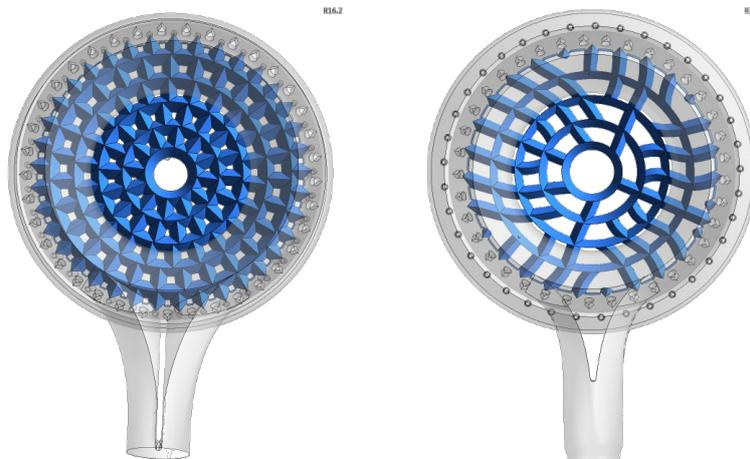
Figure 10: Studies for the design of propellant manifolds for an expander engine injector
