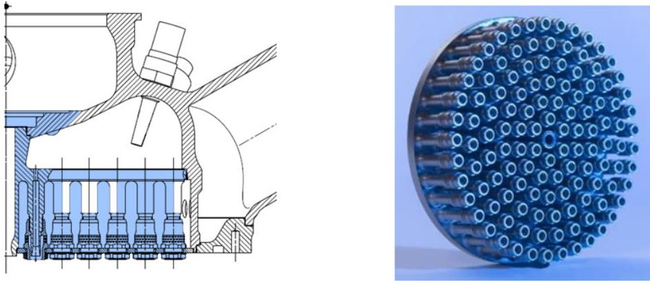
Figure 9: Vinci injector cartridge: integration concept (Left) and manufacturing sample (right)
