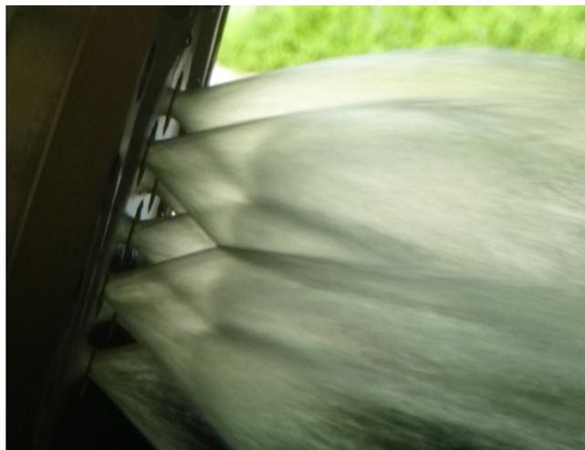
Figure 13: Flow check of full scale LNG gas generator injector
