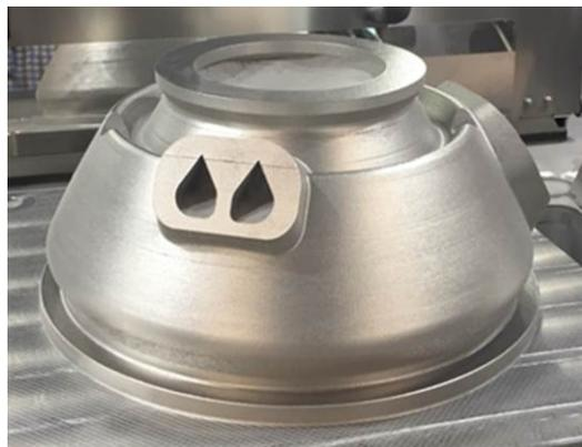
Figure 11: Full scale manufacturing demonstrator for an expander engine injector
