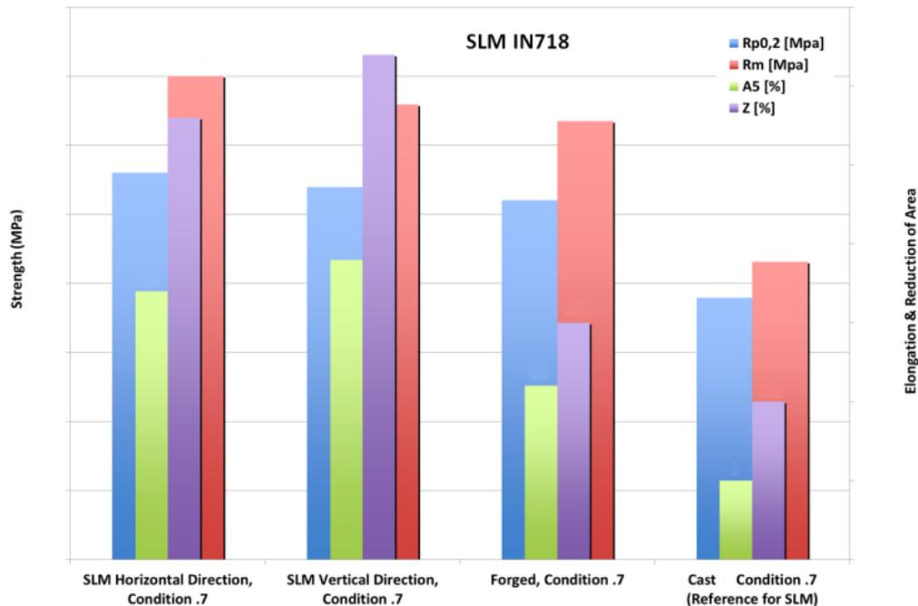
Figure 3: Results for material properties of heat-treated Inconel 718 made from additive manufacturing compared to forged and cast samples
