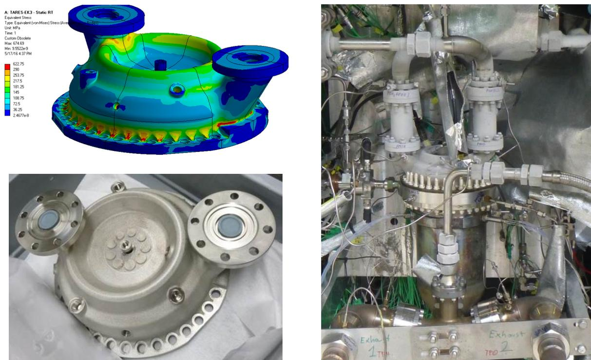
Figure 8: Redesigned gas generator injector for Vulcain 2.1 application
