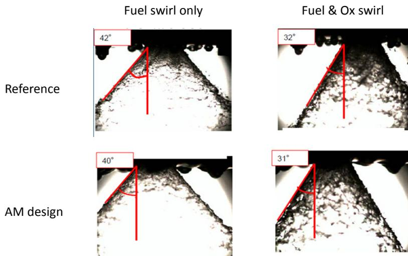
Figure 4: Flow check results for coaxial swirl injectors - comparison of spray angles from machined (top) and printed (bottom) injectors
