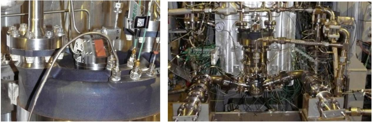
Figure 7: Additive manufactured injector installed on Vulcain 2 gas generator at P8 test facility
