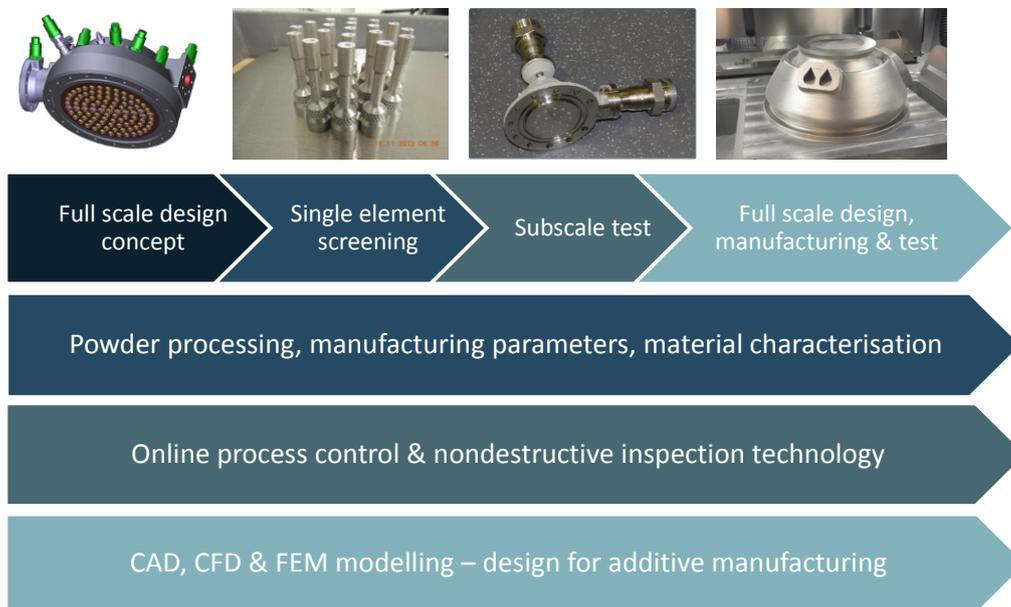
Figure 2: Additive manufacturing injector development logic
