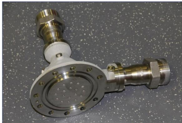
Figure 6: Subscale integral injector manufactured from stainless steel 316L
