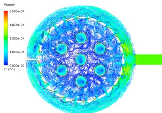
Figure 12: LOX-LCH<sub>4</sub> gas generator injector with swirl injectors: CFD simulation of fuel manifold
