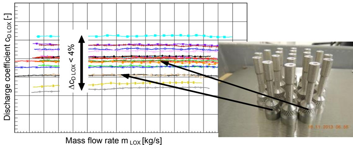
Figure 5: Discharge coefficient for additively manufactured injectors from one batch
