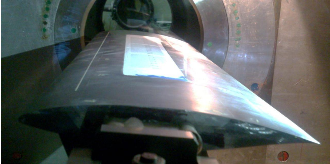
Figure 4. P-184-15SR wing equipped by longitudinal spark actuator in TsAGI T-112 wind tunnel.
