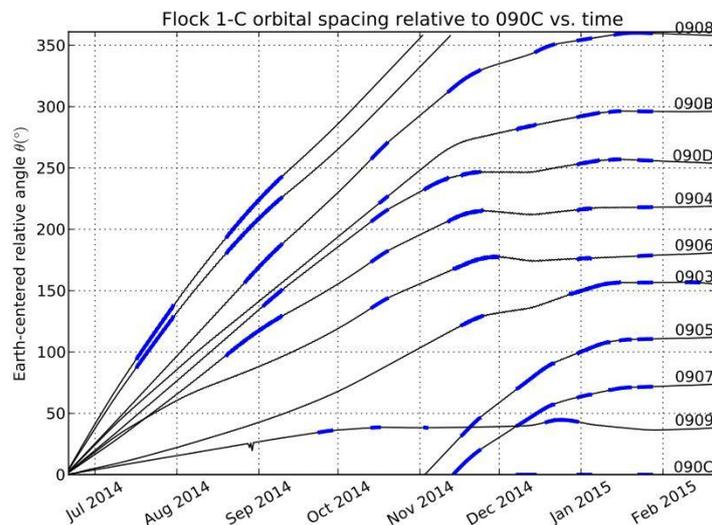
Figure 6: Actual Planet Flock 1-C position relative to the leader, 090C, measured using ranging data [2]
