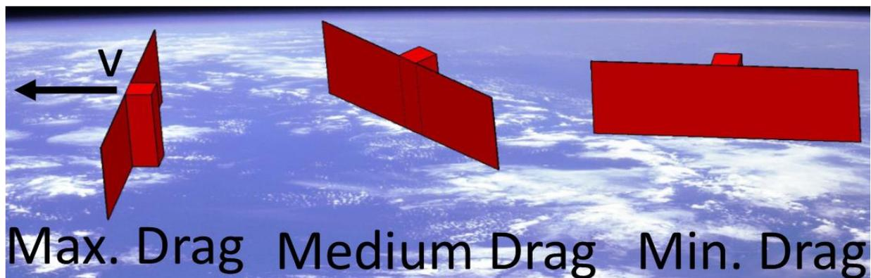
Figure 11: Spacecraft change drag acceleration without turning away from the Earth
