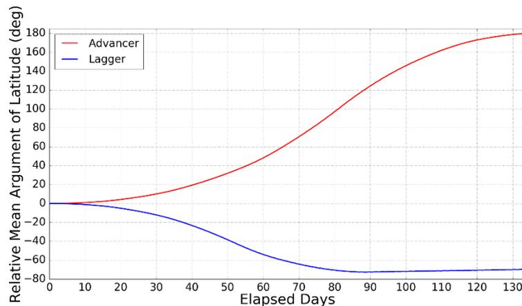
Figure 12: Simulated relative mean motion of an advancer and lagger relative to a leader spacecraft
