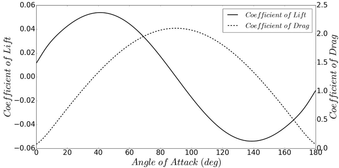
Figure 1: Variation in drag and lift with angle of attack
