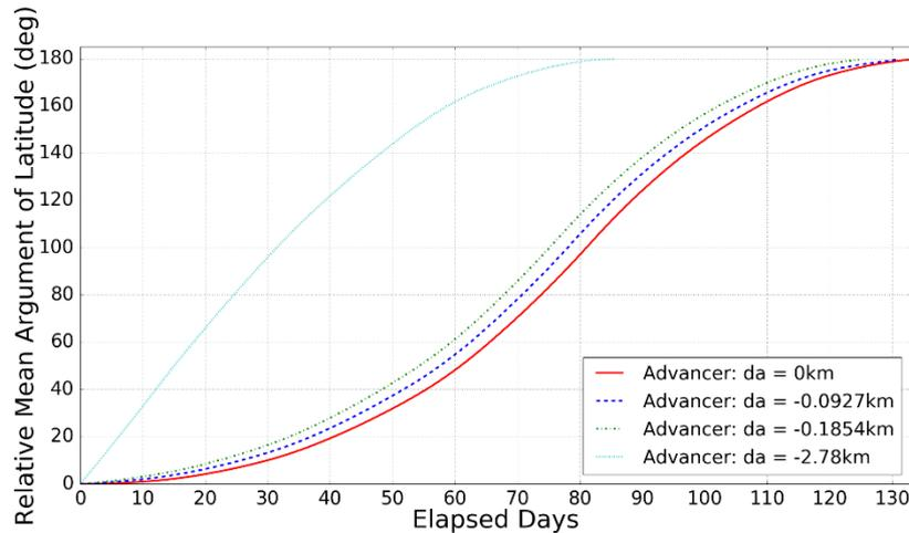
Figure 13: Difference in establishment time with subtle differences in semi-major axis ( $da$ )
