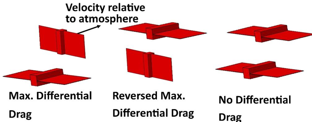
Figure 4: The set of ternary differential drag states commonly assumed in formation control algorithms
