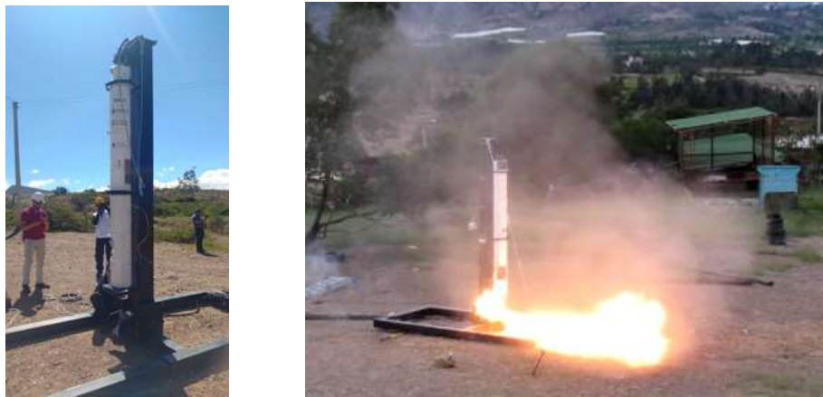
Figure 9. Left , SUA II engine mounted in UCAND II testing bench before ignition. Right , Motor firing during test.
