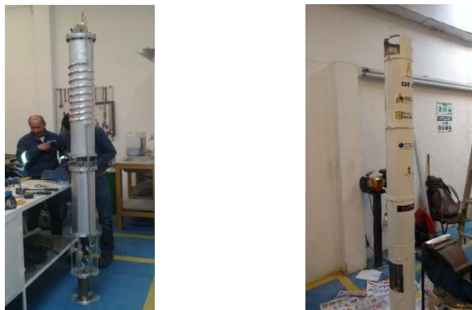
Figure 7. Finished assembly of SUA II engine and its casing test jacket.
