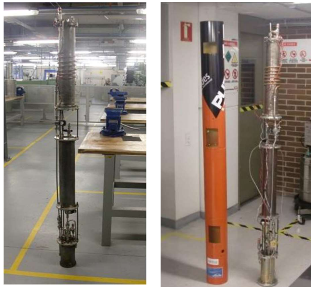
Figure 1. The PUA-1L-6S-2000N engine with its casing test jacket [8].
