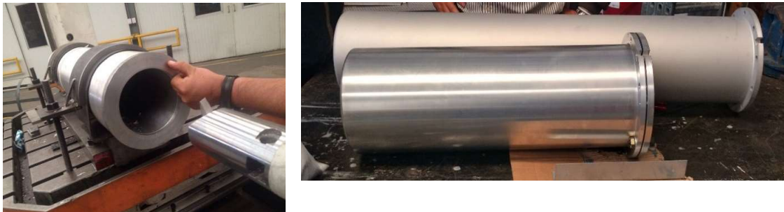
Figure 5. Left , Internal machining of the LOX tank in aluminum 6061-T6. Right , finished tanks of gasoline and LOX (anodized).
