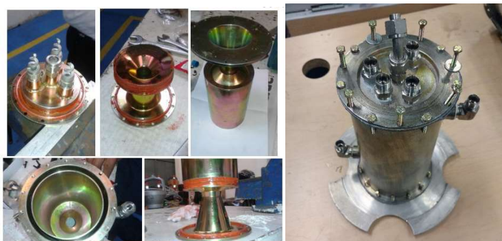
Figure 6. Left , parts and assembly process of the combustion system. Right , finished combustion system with bolts and hydraulic connections.
