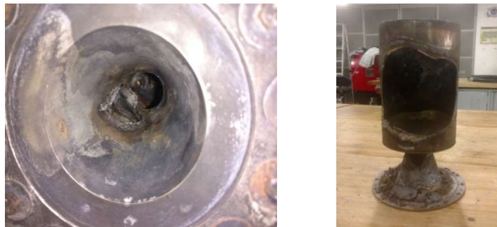
Figure 12. Left , hole caused in the throat of the nozzle. Right , damage in the combustion chamber wall.
