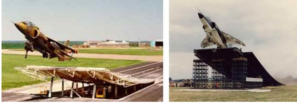
Figure 3. (Left): AV-8A trials at RAE Bedford (1977), with a 6-20° adjustable ramp. (Right), Sea Harrier FRS.1 exhibition at Farnborough Festival, 1978.
