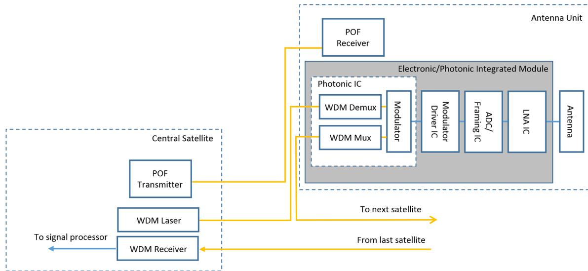
Figure 6 Schematic design of the photonic swarm front-end including the photonic system
