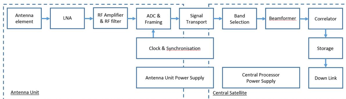
Figure 5 Scheme of general system design
