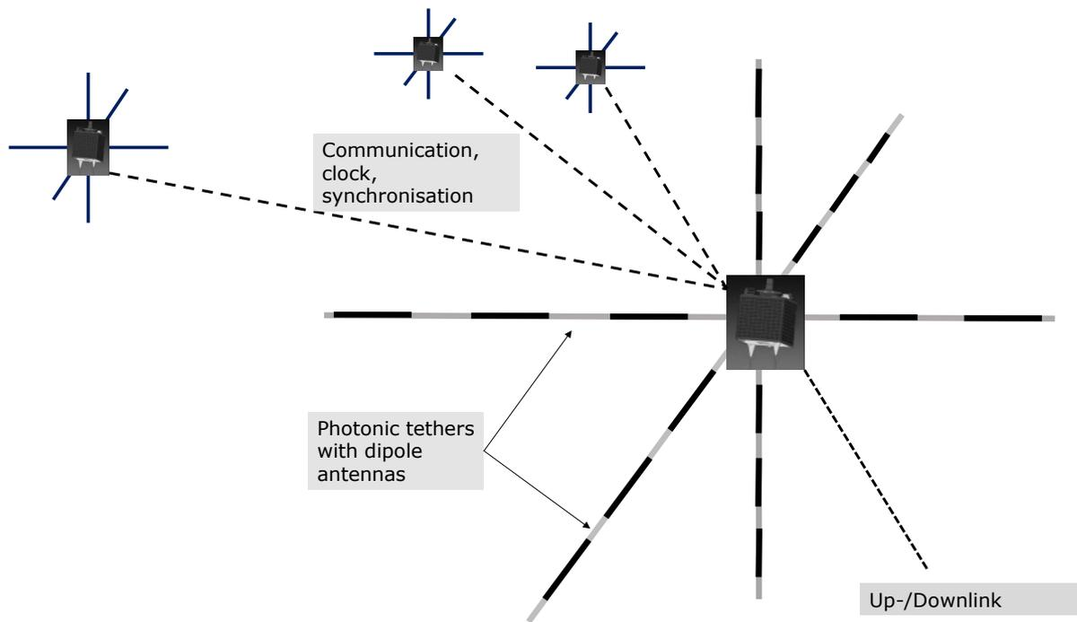
Figure 4: System concept showing the satellite and the antennas on the tethers
