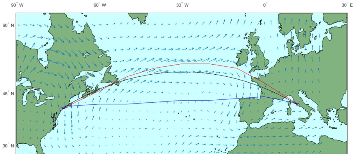
Figure 5: Optimal JFK to FCO routes (red) and optimal FCO to JFK routes (blue) for the stochastic solution.
