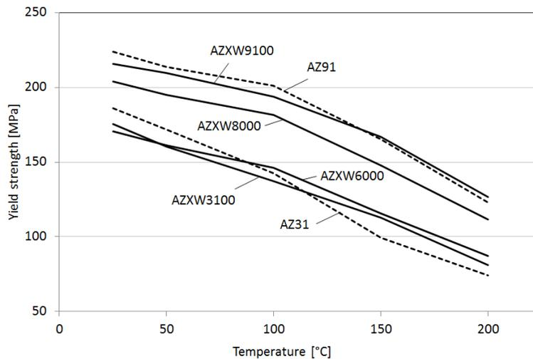
Figure 8: Temperature dependent yield strength of extrusion pressed alloys
