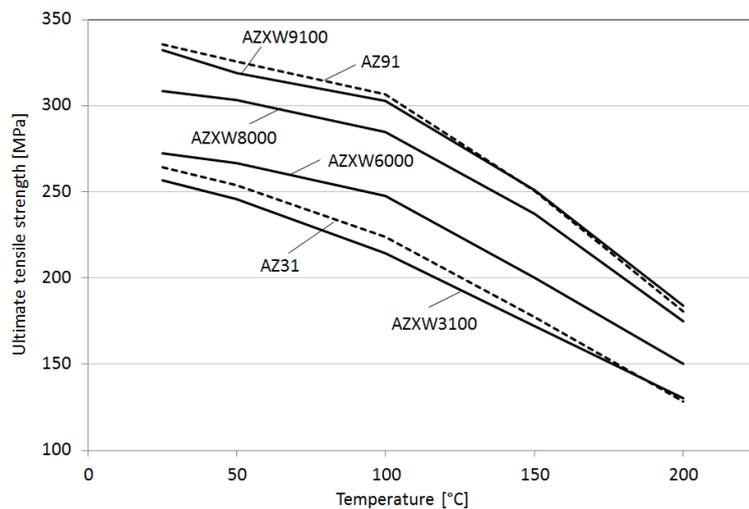
Figure 9: Temperature dependent ultimate tensile strength of extrusion pressed alloys
