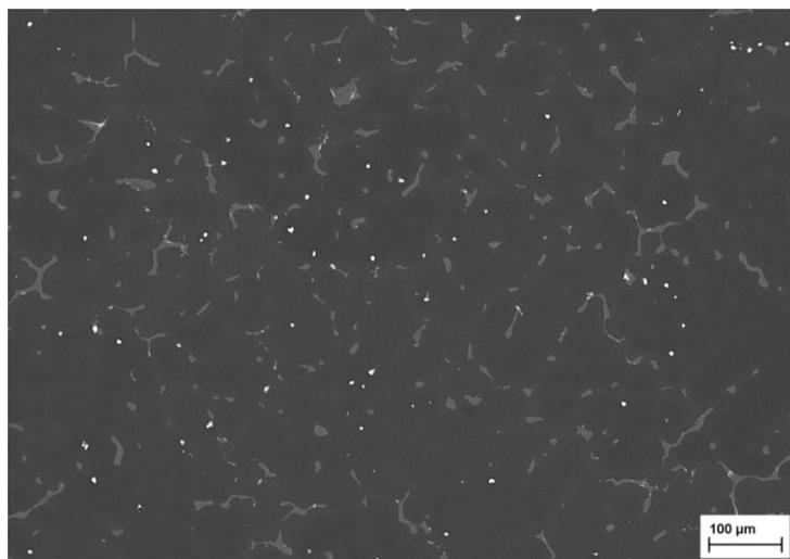
Figure 3: Microstructure of AZ91 alloy – as cast condition
