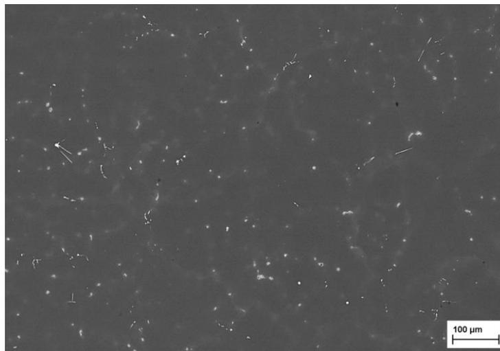
Figure 2: Microstructure of AZ31 alloy - as cast condition
