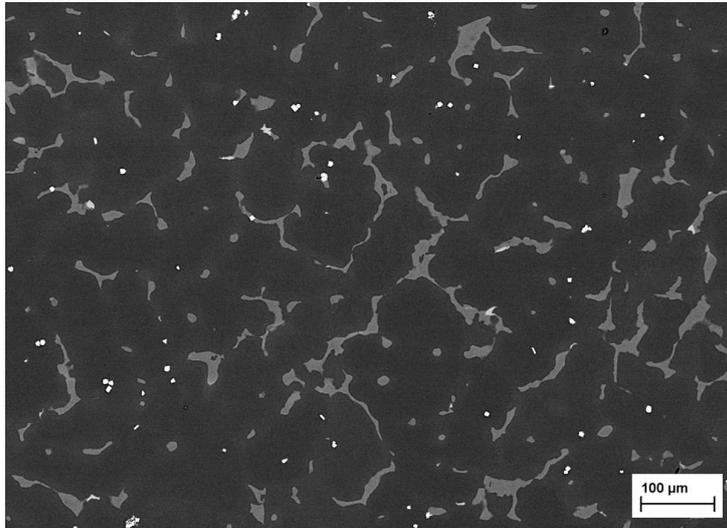
Figure 5: Microstructure of AZXW9100 alloy – as cast condition
