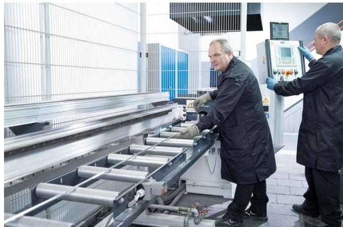
Figure 1: Extrusion pressing of Ø 10 mm profiles
