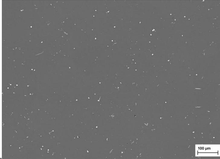
Figure 4: Microstructure of AZ91 alloy – heat treated condition
