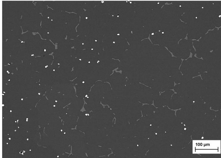
Figure 6: Microstructure of AZXW9100 alloy – heat treated condition
