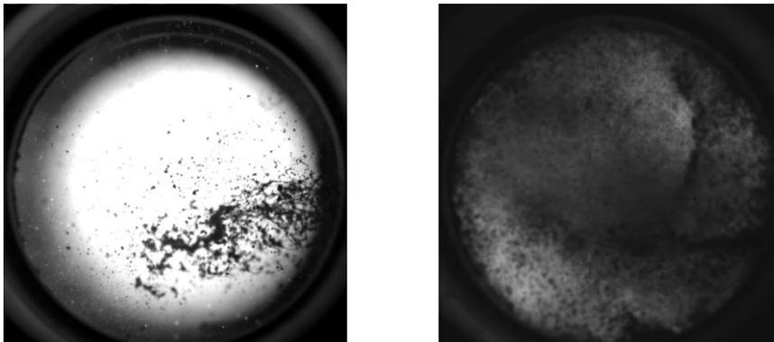
Figure 2: Initiation of gel injection (left) and accumulation of combustion products after 1.5 s (right) (snapshot from high speed video of preliminary test)
