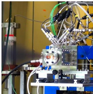
Figure 4: First hot fire test of new gel rocket combustion chamber with optical access (windows replaced by dummies)
