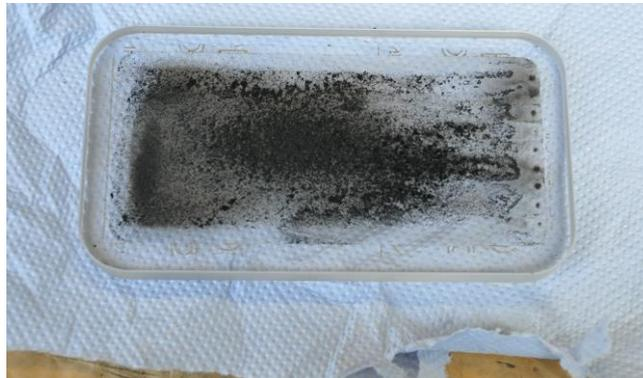
Figure 10: Soot on dismantled sapphire window after three consecutive tests with injector "B" (flow direction from right to left)
