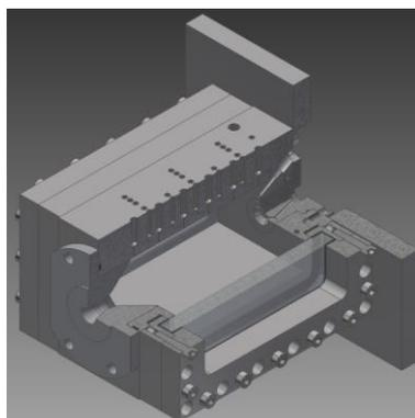
Figure 3: Sketch of new rectangular gel rocket combustion chamber with optical access (3/4 cut-out, simplified)
