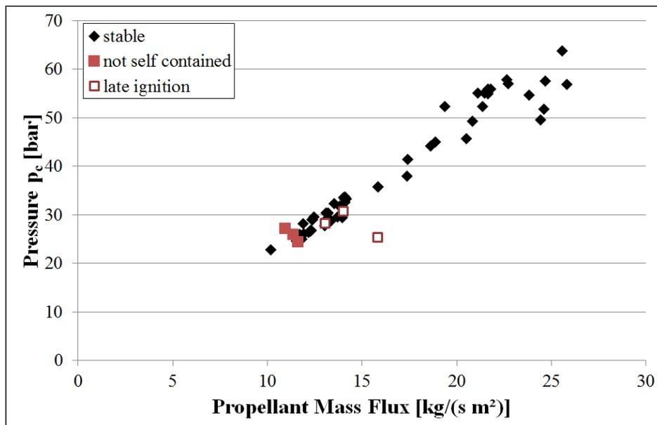
Figure 6: Stability and self-contained combustion
