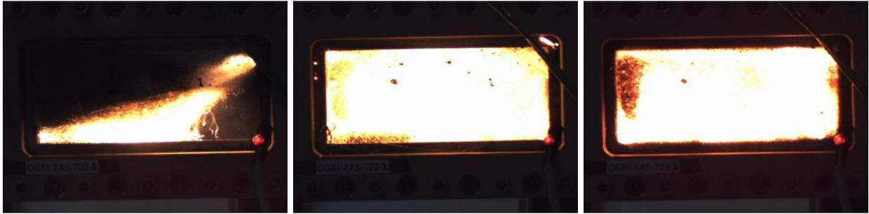
Figure 8: Ignition, startup and nominal operation recorded with general purpose industrial camera (flow direction from right to left)
