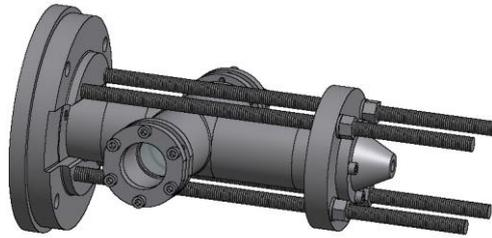
Figure 1: Sketch of gel combustion chamber with round windows used for preliminary tests
