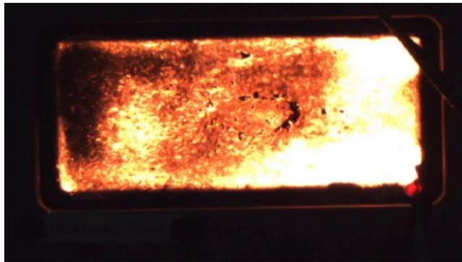
Figure 9: Depositions on sapphire window during test with injector "A" (flow direction from right to left)
