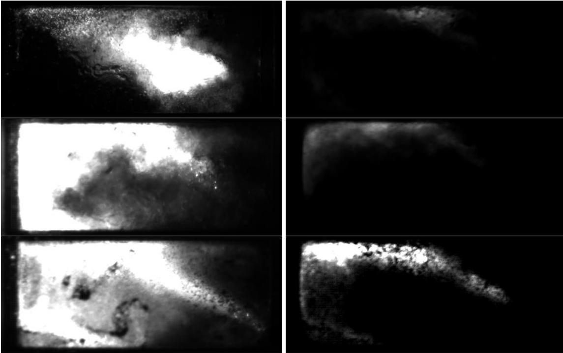
Figure 11: First gel ignition, snapshots from high speed camera recordings, flow direction from right to left (left hand side: unfiltered, 1/720000 s exposure time; right hand side: CH\* filter, 1/10000 s exposure time)
