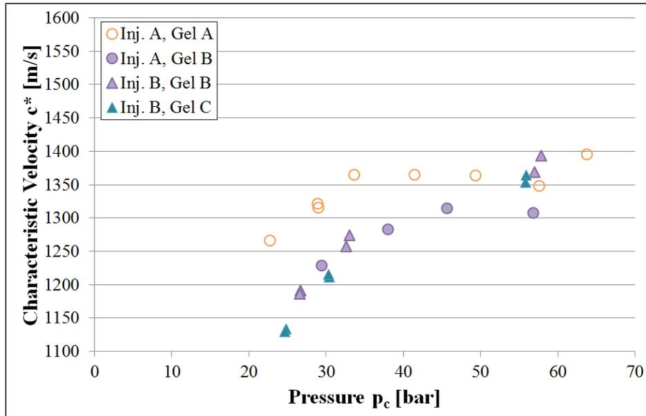
Figure 7: Combustor performance for different gel propellants and two injector elements
