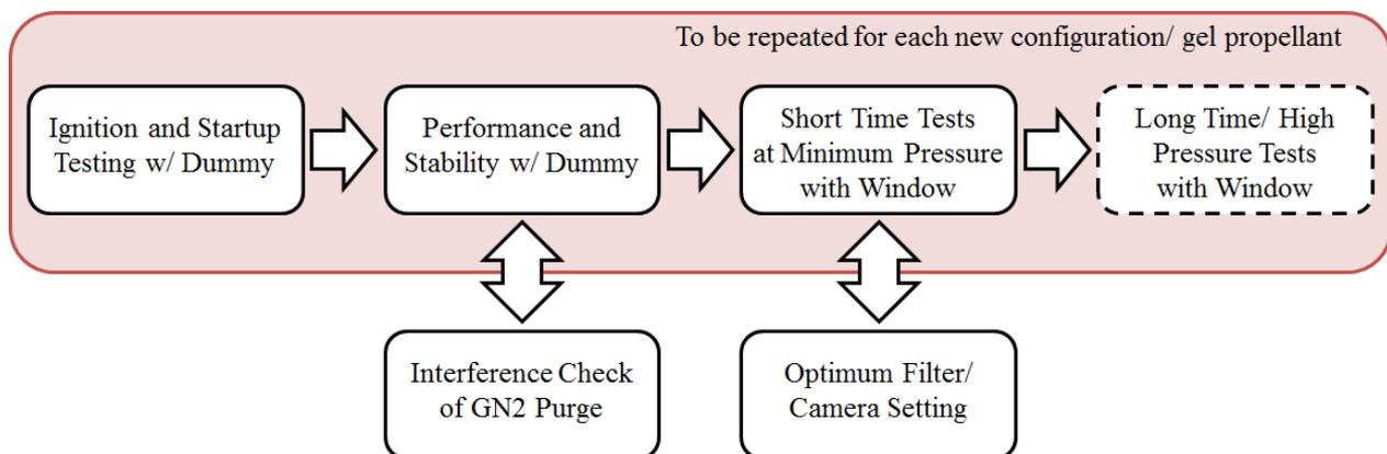
Figure 5: Test methodology for testing the gel rocket combustion chamber with optical access
