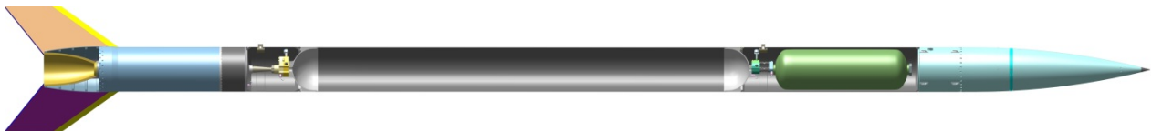
Figure 14: The design of the Nucleus sounding rocket demonstrator ( Nammo )
