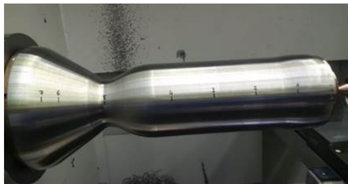
Figure 6: ID#1 Combustion chamber, with NiCo jacket ( ARIANE GROUP GmbH )
