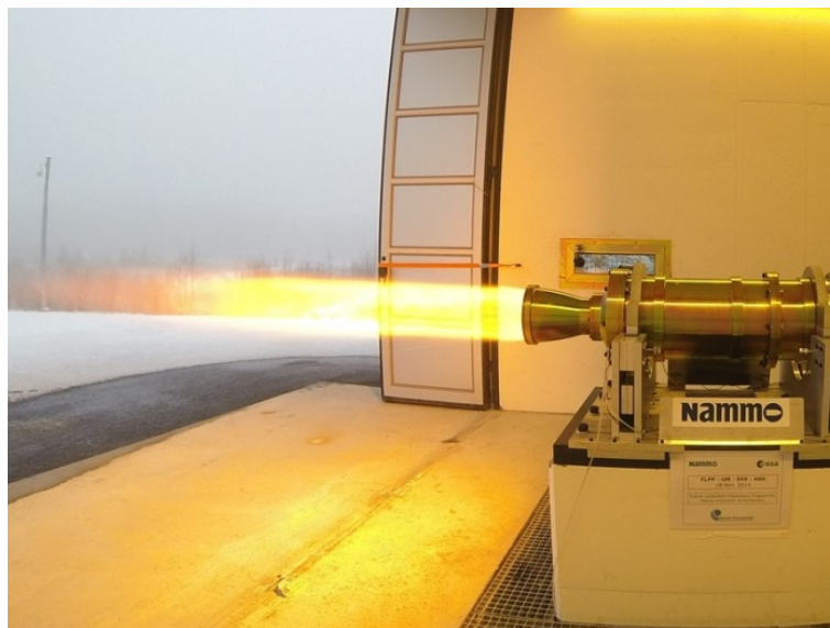
Figure 12: Hybrid engine demonstrator hot fire test in heavy wall configuration ( Nammo )
