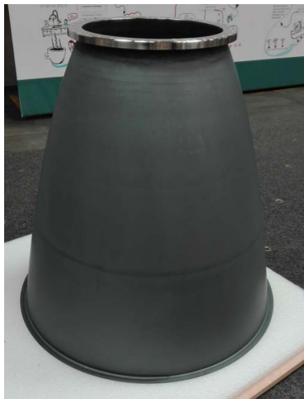
Figure 2: Nozzle demonstrator with welded flange ( Franke Industrie AG, Ariane Group GmbH )
