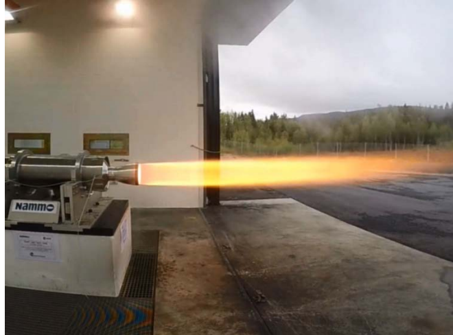
Figure 13: Hybrid engine demonstrator hot fire test in flight weight configuration ( Nammo )
