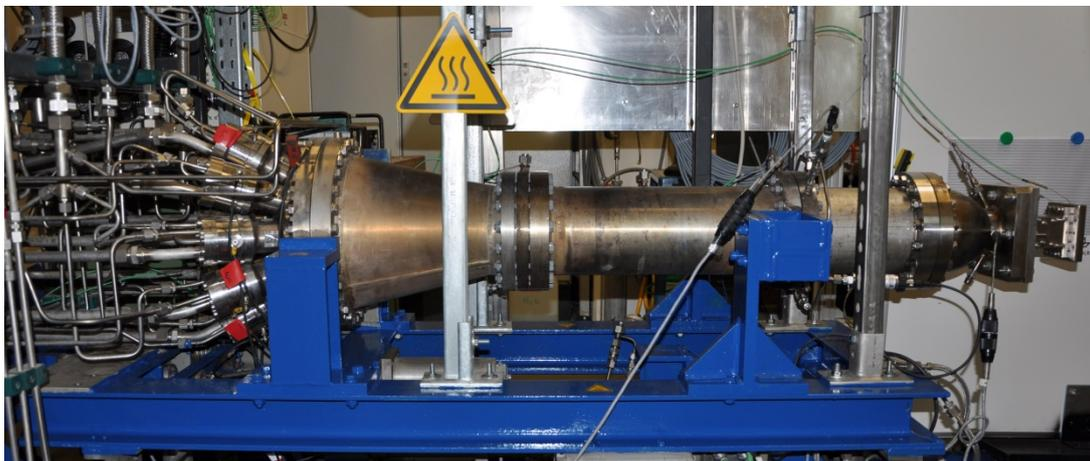
Figure 1: Air Vitiator with Attached Supersonic Nozzle and Scramjet Model Combustion Chamber
