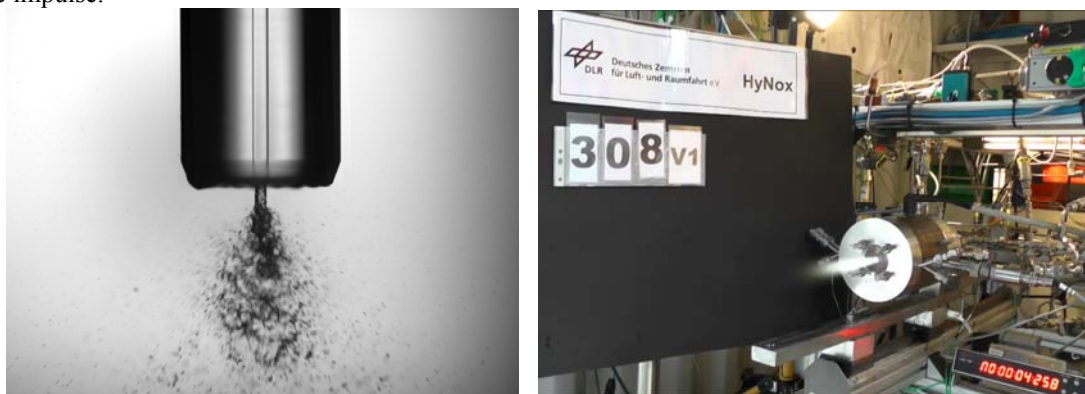
Figure 14: Left: Shadowgraph image of flash vaporization. Right: HyNOx model combustor at M11.5.
