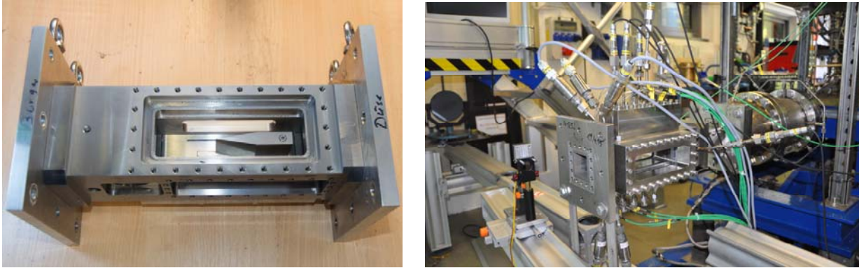
Figure 16: Scramjet model combustor for the investigation of transpiration cooling processes. Left: combustor without windows. Right: Experimental setup with combustor at M11.1.
