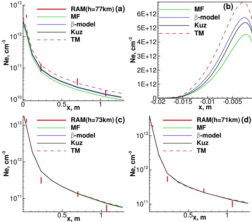
Figure 8: Comparison of the number density of electrons with experimental data for  $h=77$  km (a),  $h=73$  km (c),  $h=71$  km (d). Distributions of the electron density along the stagnation line for  $h=77$  km (b) predicted by different models.
