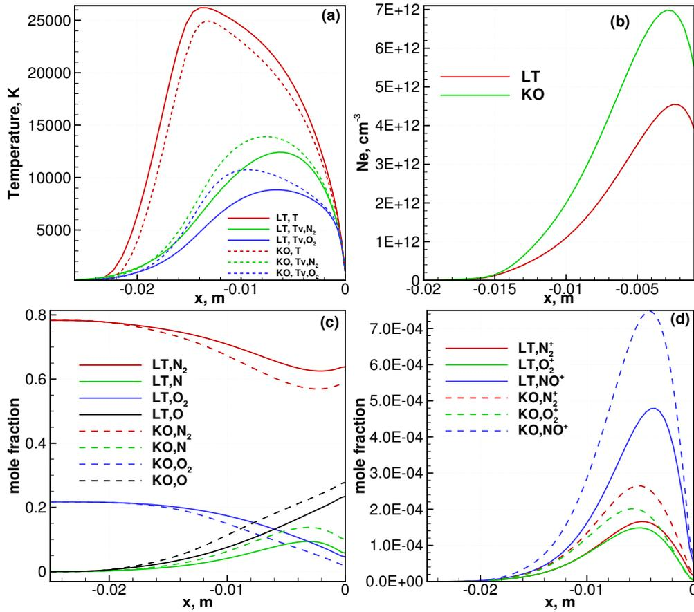
Figure 3: Distributions of translational-rotational and vibrational temperatures of molecular nitrogen and oxygen (a), electron density (b), and molar fractions of neutral (c) and charged (d) components of the mixture along the stagnation line predicted by different models of vibrational relaxation for  $h=77$  km.
