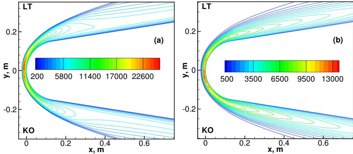
Figure 2: Comparison of the fields of translational-rotational (a) and vibrational (b) temperatures predicted by different models of vibrational relaxation for  $h=77$  km.
