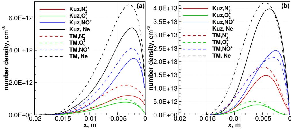
Figure 7: Distributions of the number density of charged particles along the stagnation line computed with the use of the Kuznetsov and Treanor–Marrone dissociation models for  $h=77$  km (a) and  $h=71$  km (b).
