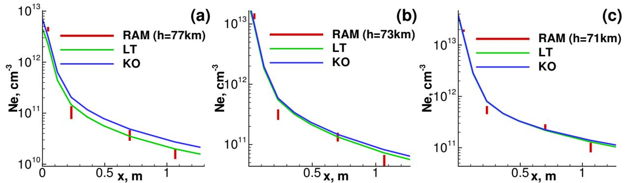
Figure 4: Comparison of the predicted maximum electron density with flight experiment data for  $h=77$  km (a),  $h=73$  km (b), and  $h=71$  km (c).
