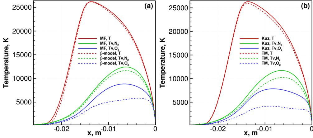
Figure 5: Distributions of translational-rotational and vibrational temperatures of molecular nitrogen and oxygen along the stagnation line ( $h=77$  km) predicted by different dissociation models: Macheret–Fridman and  $\beta$ -model (a), Kuznetsov and Treanor–Marrone models (b).
