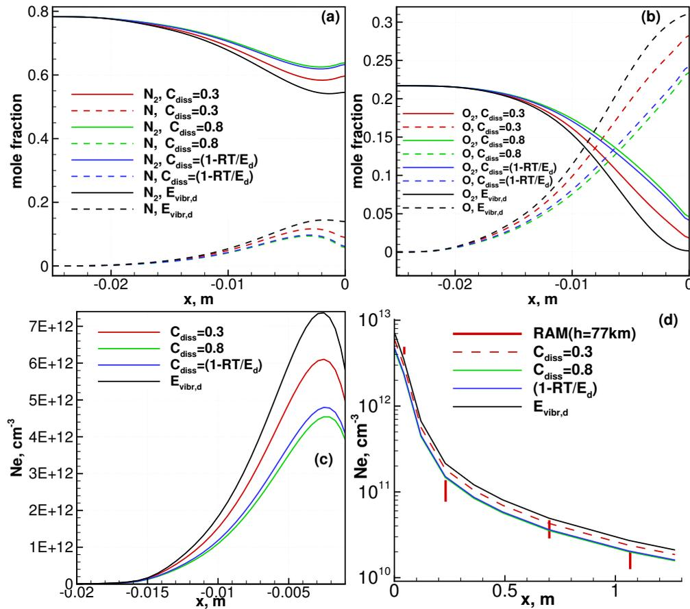
Figure 9: Distributions of the molar fractions of nitrogen (a) and oxygen (b) and of the number density of electrons (c) along the stagnation line and comparison with experimental data for  $h=77$  km. The computations are performed for different values of  $R_d^{\text{vibr,chem}}$ .
