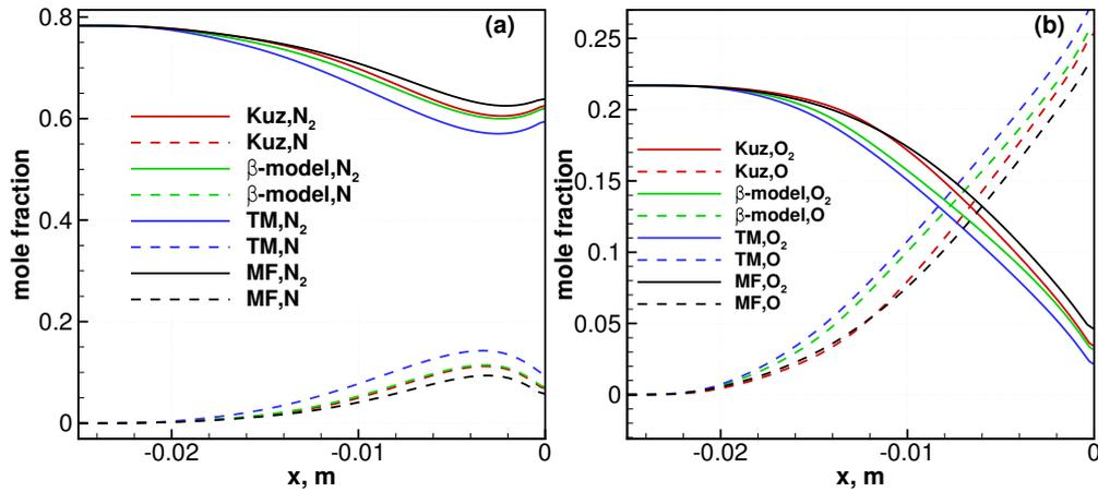
Figure 6: Distributions of the molar fractions of nitrogen (a) and oxygen (b) along the stagnation line ( $h = 77$  km) predicted by different dissociation models: Macheret–Fridman,  $\beta$ -model, Kuznetsov, and Treanor–Marrone models.
