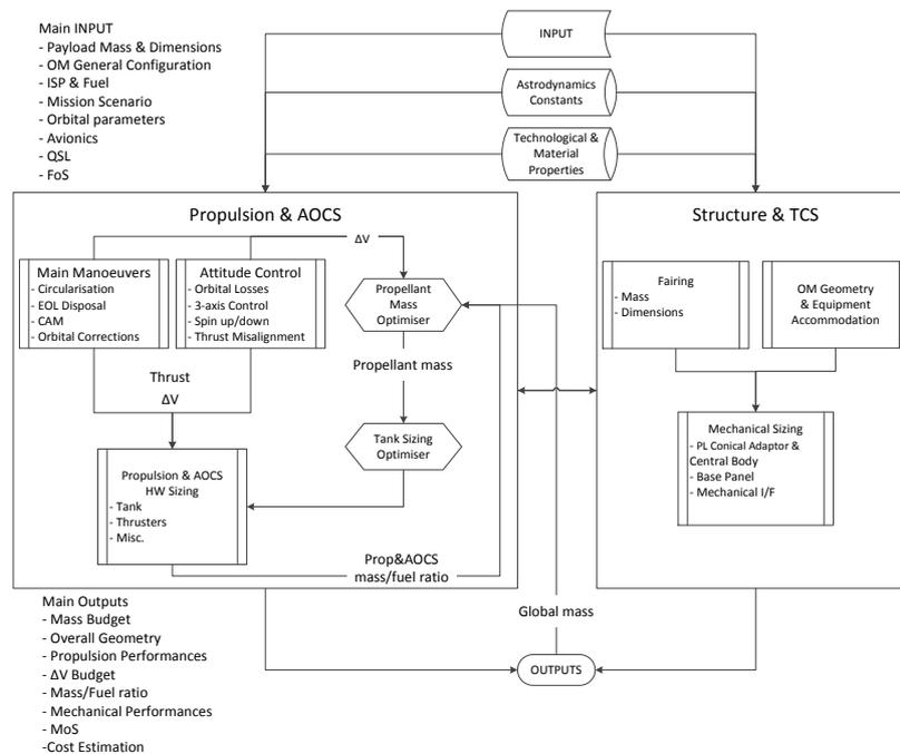
Figure 5: ALTAIR OM System Optimisation Design Loop
