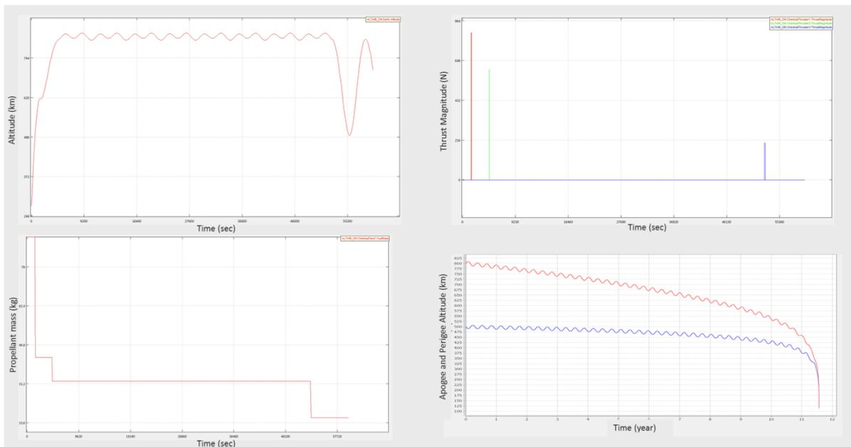
Figure 16: OM altitude, thrust magnitude, propellant mass consumption and apogee/perigee altitude evolution in function of time
