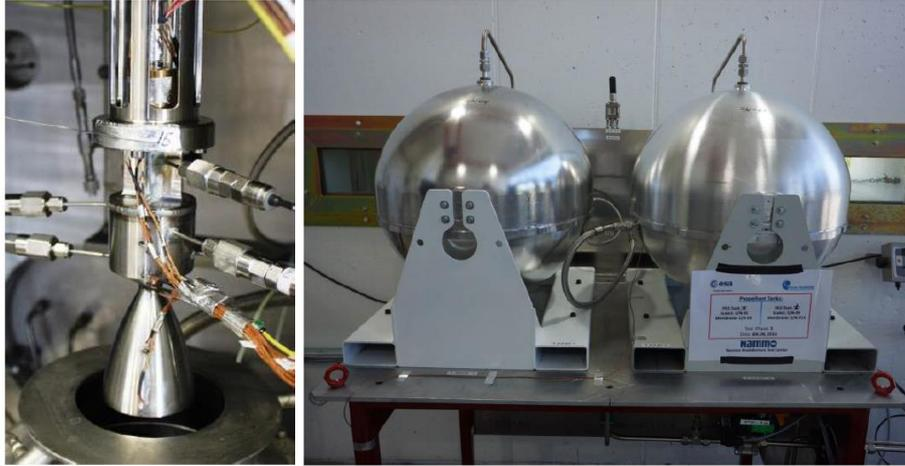
Figure 12: Early design of Nammo's 200 N flight-weight thruster for Ariane 5 ME in a vacuum chamber test cell (left) and Nammo's propellant tanks for hydrogen peroxide (right) (Source: Nammo)
