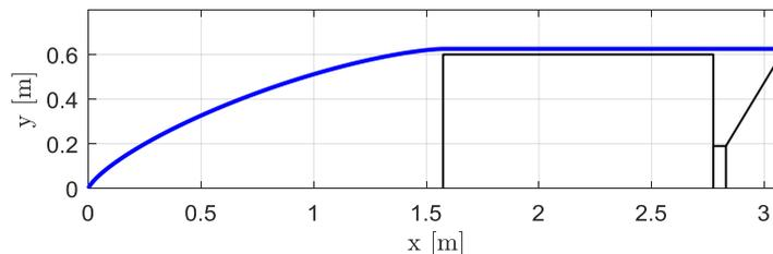
Figure 13: Preliminary fairing geometry
