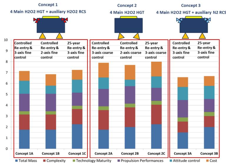
Figure 7: OM propulsion architecture, attitude control and EoL disposal strategy trade-off synthesis
