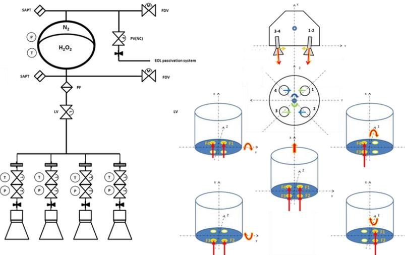
Figure 11: ALTAIR OM Propulsion System Scheme (left) and attitude control thruster mounting and activation strategy (right)
