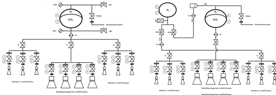
Figure 4: Example of OM potential propulsion system architecture.
