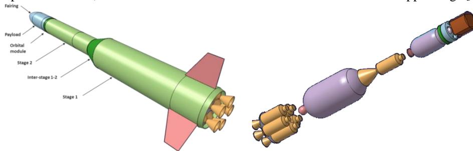
Figure 2: General architecture of the ALTAIR launch vehicle
