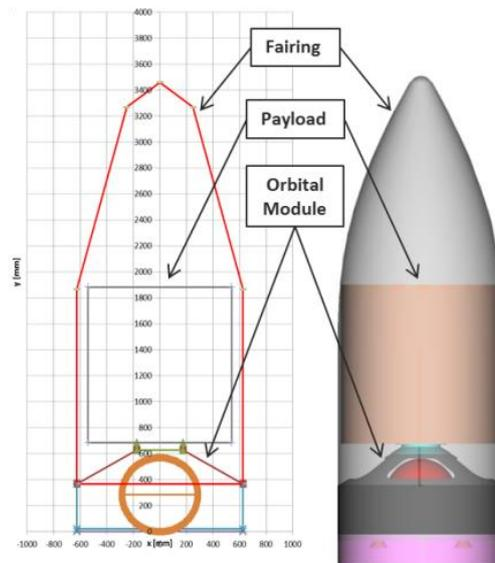
Figure 8: Current status of ALTAIR ORBITER Configuration.
