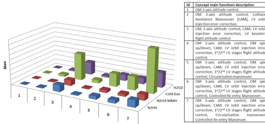
Figure 6: Trade-off synthesis on OM mass Vs Functions Vs Propellant technology
