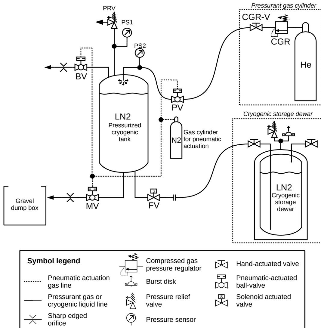
Figure 5: Feed system schematics of the test setup used during the validation tests.
