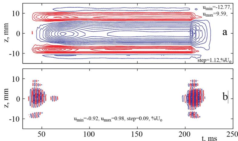
Figure 3: Contours of velocity fluctuations in  $z$ - $t$  plane at  $y=0.8$  mm ( $u_{\max}$ ),  $x=200$  mm, (a) – not filtered; (b) – filtered in a frequency band 200-350Hz
