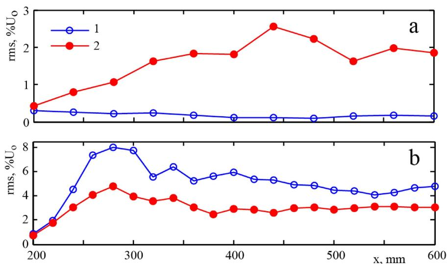
Figure 7: Distribution of the wave packets amplitude downstream, at leading (1) and trailing (2) front,  $z=0$  mm  $y=y_{U_{\max}}$ ; (a) – for the  $U_0=16$  m/s, (b) –  $U_0=18$  m/s.
