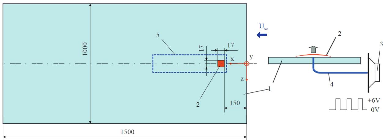
Figure 1: Set-up, dimensions in mm; 1–plate, 2–membrane, 3–loudspeaker, 4–pipeline, 5–measurement area.
