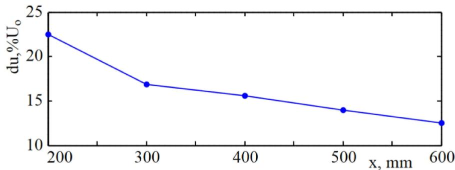
Figure 6: Distribution of the localized streak amplitude downstream at  $U_\infty=16$  m/s,  $y=y_{U_{\max}}$
