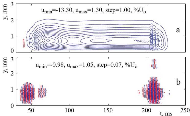
Figure 4: Contours of velocity fluctuations in  $y$ - $t$  plane at  $z=0$  mm,  $x=200$  mm, (a) – not filtered; (b) – filtered in a frequency band 200-350Hz
