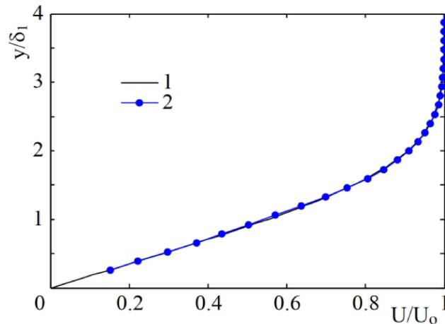
Figure 2: Mean velocity profiles of theoretical Blasius (1) and measured base flow (2),  $U_\infty = 16$  m/s,  $x=200$  mm.
