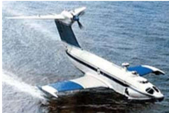
Figure 1: Assault ekranoplane "Orlyonok" with plane-like configuration of 140 ton weight
