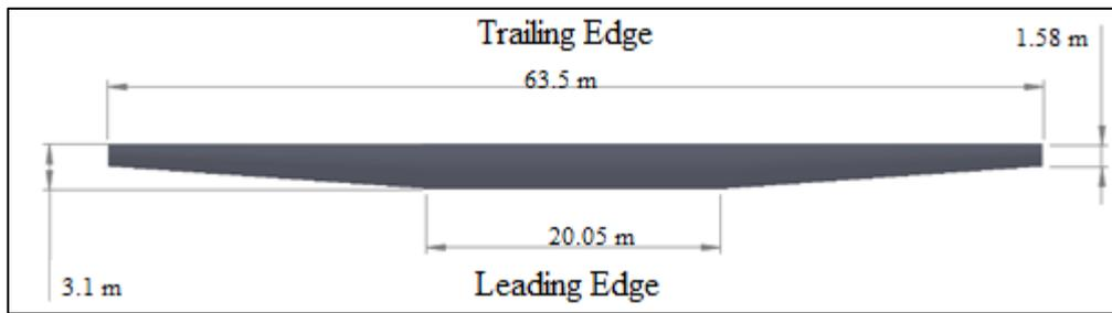
Figure 3 Details of wing geometry
