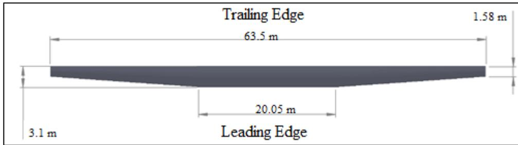
Figure 3 Details of wing geometry
