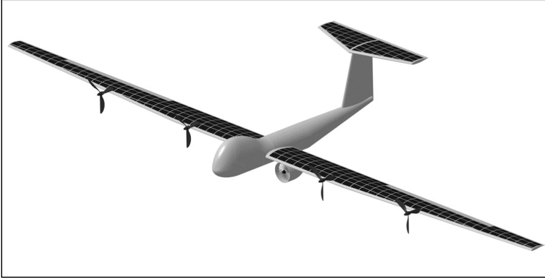
Figure 6 Isometric view of the aircraft
