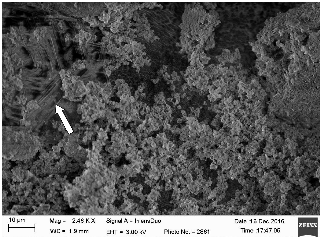
Figure 3: The SEM-image of the CCP particles sediment for the propellant 18B with boron only (sample cleaning ). There are the scaly formations with the terraces of growth typical of crystallization (marked with arrow).
