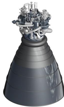
Figure 2: Outside drawing of the second stage engine of H3 launch vehicle; LE-5B-3
