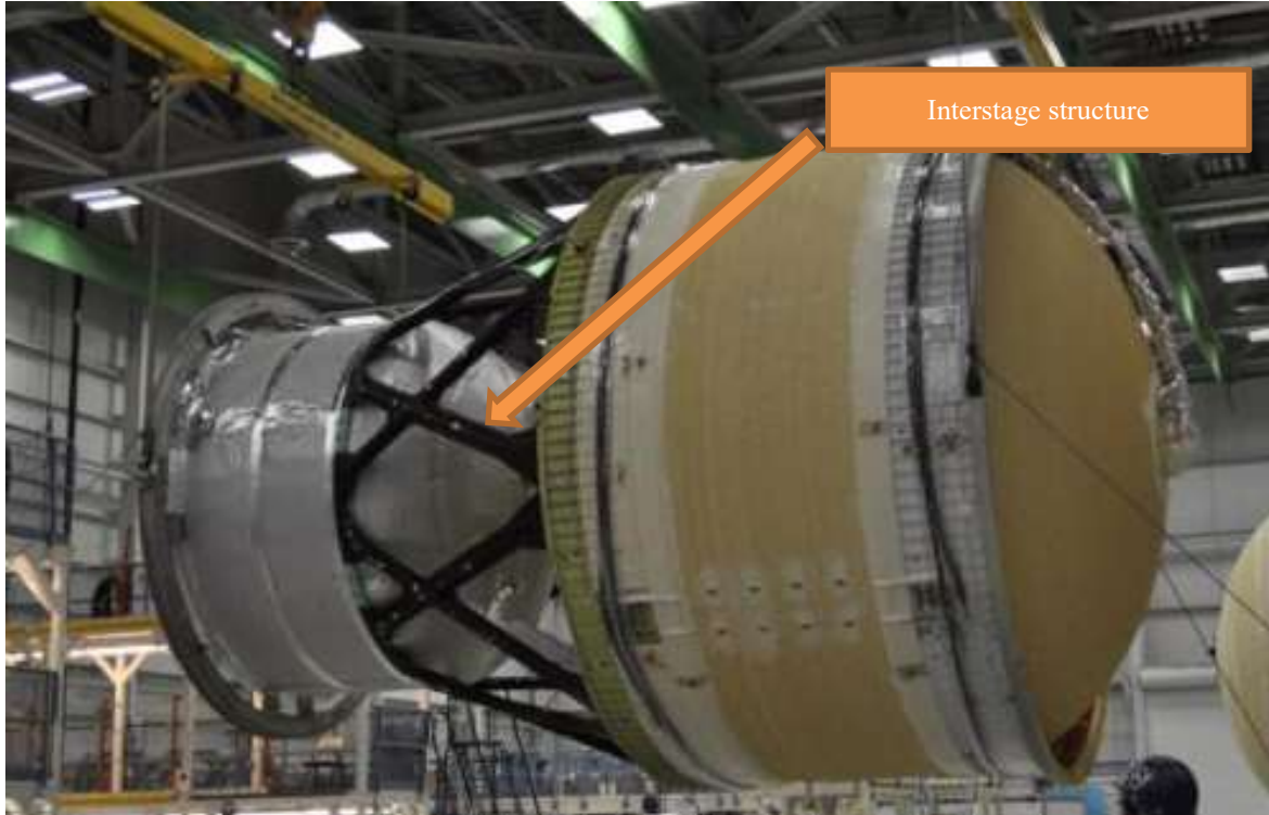
Figure 1: ICPS picture showing the location of the interstage structure. Image credit: ULA
