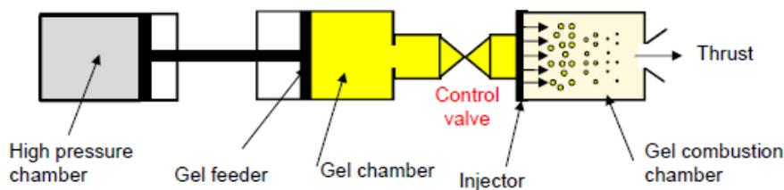
**Figure 1: Principle of operation of a GRM**
