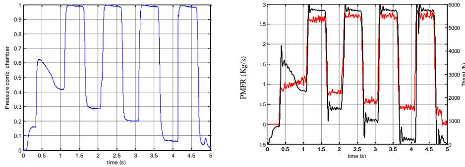
**Figure 6a-b: GRM-02 Combustion chamber pressure (a), PMFR and Thrust (b)**
