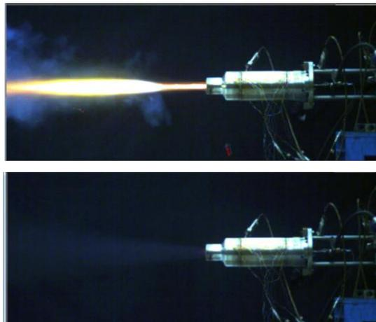
**Figure 7: High speed photos during ignition and after ignition end**
