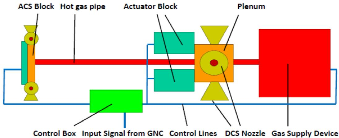
Figure 10: Principle sketch of the main building blocks of a DACS.
