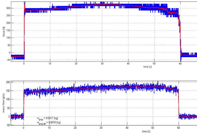
Figure 4a-b: GRM-001 (300 N GRM) thrust and PMFR
