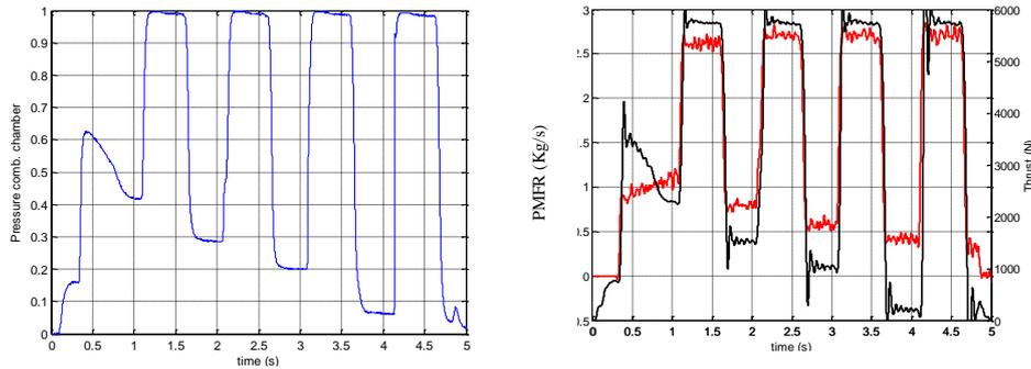
**Figure 6a-b: GRM-02 Combustion chamber pressure (a), PMFR and Thrust (b)**
