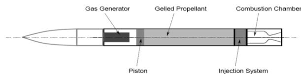
Figure 5: gel propellant rocket motor for a conventional missile
