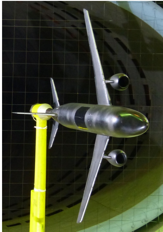
Figure 1. Fully iced aircraft model installed on the tail support strut in the wind tunnel test section.
