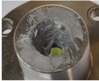
Figure 6: Propellant residue in nozzle after pilot flame ignition test
