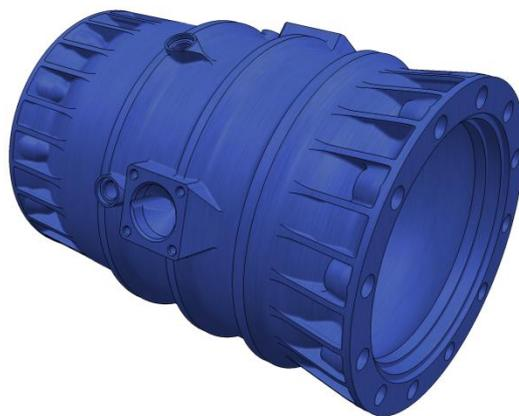
Figure 10: HCV housing (to be manufactured by ALM process)
