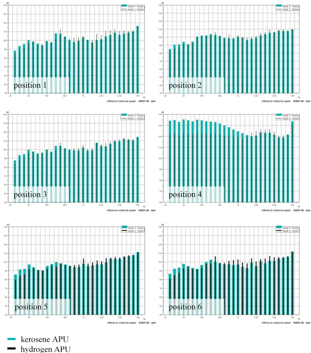
Figure 9: Comparison of the third-octave band spectra's of hydrogen and kerosene run
