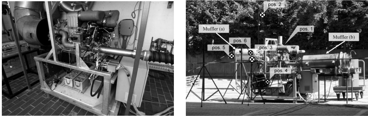
Figure 1: GTCP 36-300 at exhaust emission test stand (left) and during free-field noise measurement (right)
