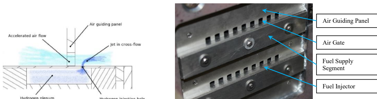
Figure 2: Section view of a Micromix combustor
