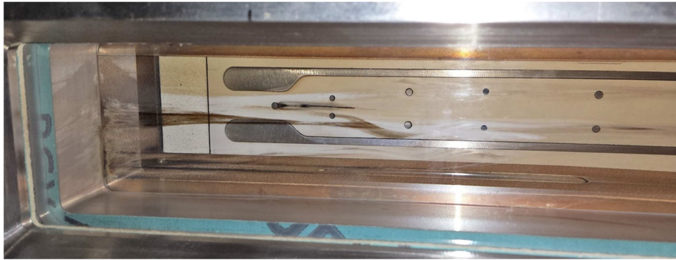
Figure 6: Plasma/injection module connected to the supersonic combustor
