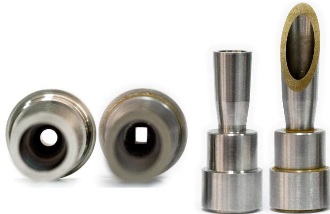
Fig. 2.2. Pairs of photographs of the axisymmetric nozzle (left) and beveled nozzle with a rectangular throat (right) in two projections
