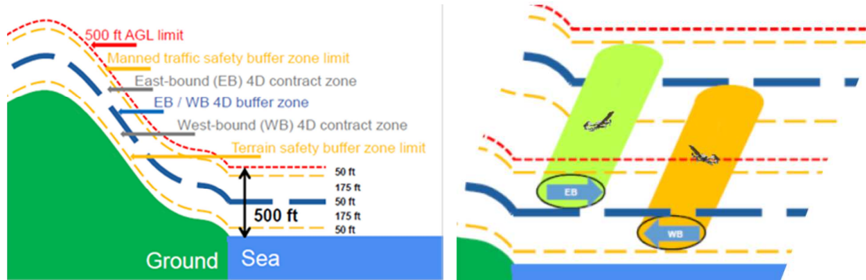
Figure 1: Semi-circular rule for RPAS VLL operations and perspective view of the RPAS traffic.
