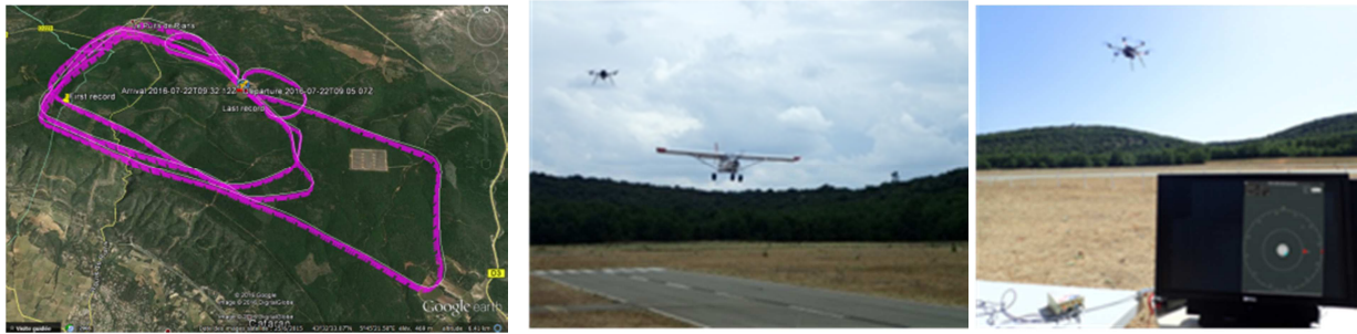
Figure 4: Illustration of first flight tests, showing the flown intruder trajectories, a conflict situation between the RPA and the intruder, and the LLRTIM ground segment with the display intended for use by the remote pilot.
