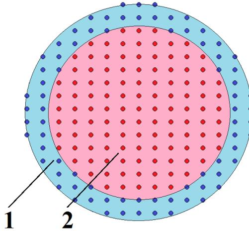
Figure 2: The model of droplet flow consisting of core and periphery. The numbers denote: 1 - the periphery of the flow, 2 - the core of the flow.
