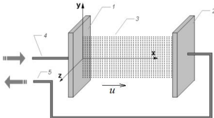
Figure 1: Liquid droplet radiator. 1 - The generator of drop flow; 2 – Hydro-collector; 3 - Droplet flow; 4, 5 - The pipeline. The velocity of droplets  $u$  is directed along the axis  $x$ .
