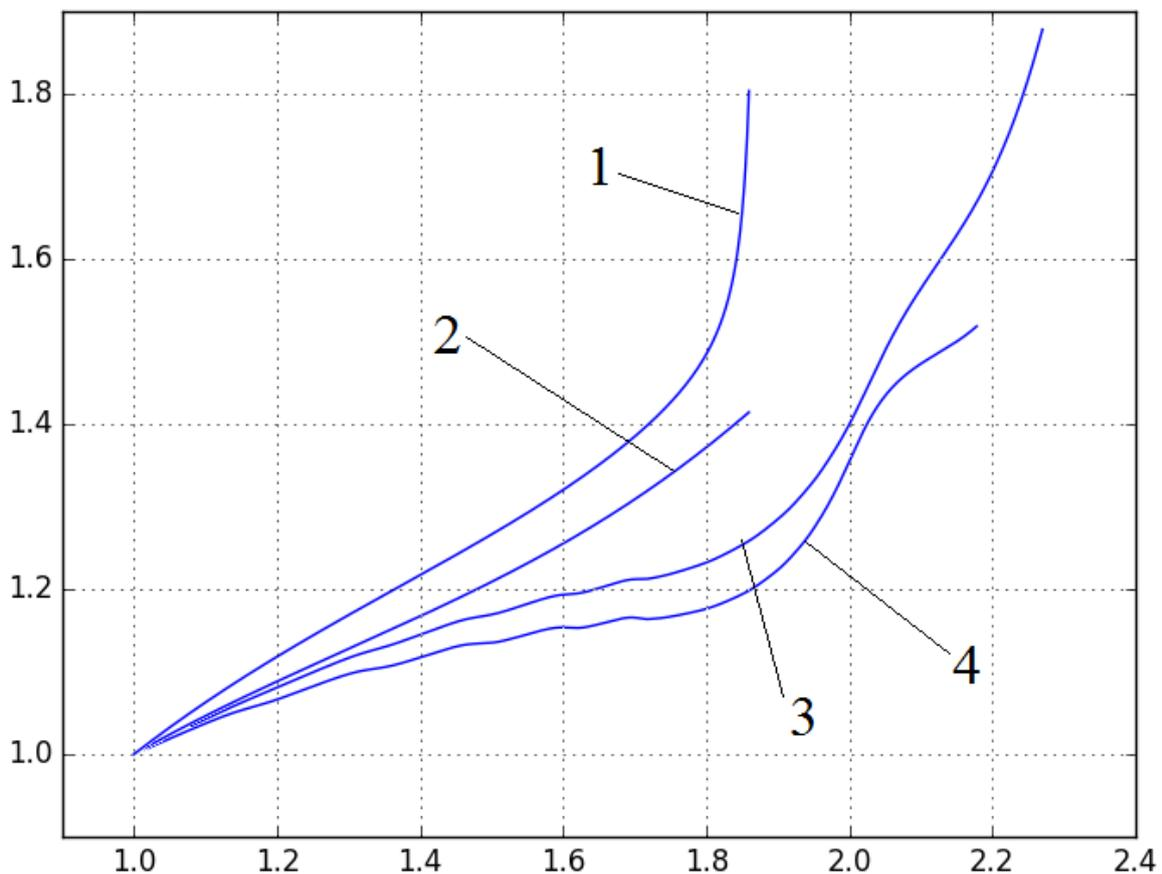
Figure 4: Numerical solution of the cooling problem (20). On the abscissa axis  $\tau_c$  is plotted, and  $\tau_p$  is plotted along the ordinate axis. 1 - Only solar radiation is considered; 2 - Both solar radiation and distant radiation interactions weren't taking into account; 3 - both solar radiation and distant radiation interactions are considered; 4 - only distant radiation interactions are taken into account. The initial condition is:  $\tau_c = \tau_p = 1$ .
