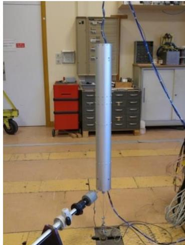
Figure 9 – Suspension and shaker during the laboratory tests
