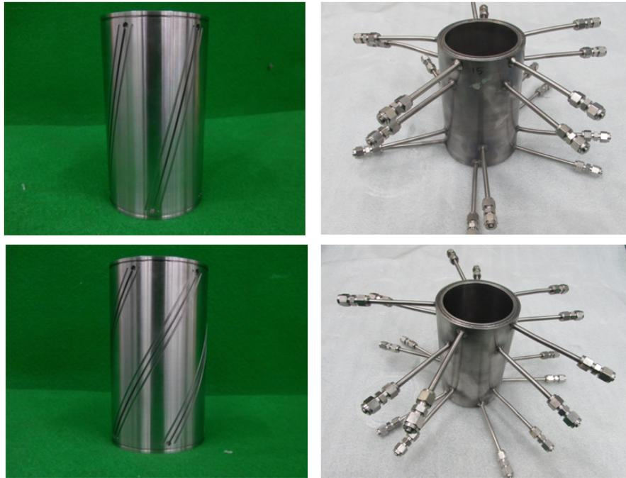
Figure 2: Photographs of the manufactured helical cooling channel (upper: 15° lower: 30°)
