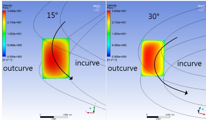
Figure 5: Velocity components in the channel at 30 m/s by CFD analysis (left : 15°, right : 30°)
