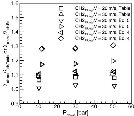
Figure 7: Ratio of friction coefficient measured from the present tests by analytical friction coefficients at CH2
