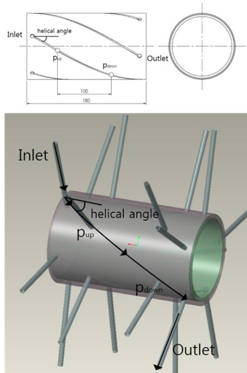
Figure 1: 2D drawing and 3D model of the helical cooling channel
