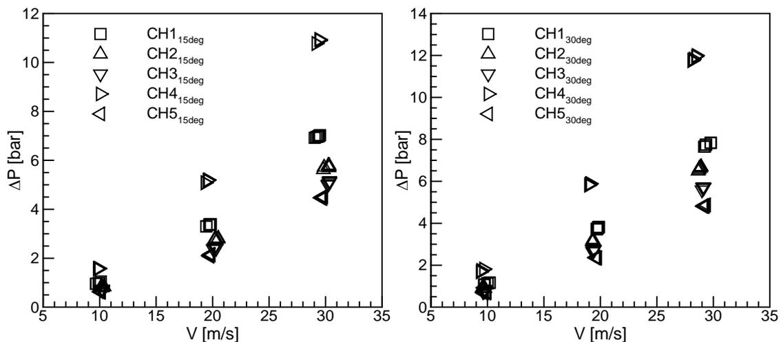
Figure 4 Pressure loss data as a function of the coolant velocity (upper: 15° lower: 30°)
