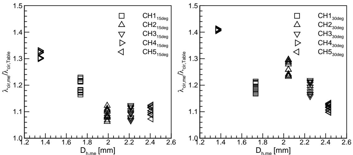
Figure 6 Ratio of friction coefficient measured from the present tests by friction coefficient obtained from the Table (upper: 15° lower: 30°)
