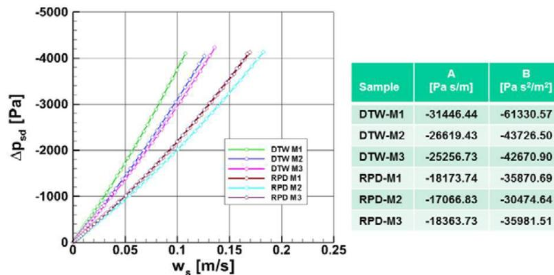
Figure 6: Pressure loss characteristics of six test samples with varying buildup of hybrid layers
