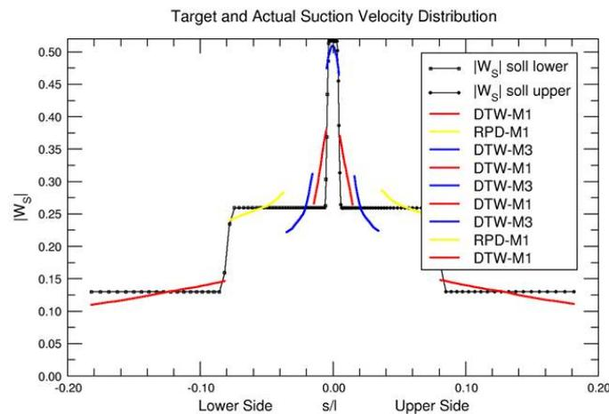
Figure 7: Target and actual suction velocity vs. arc length along contour of cross section DV2
