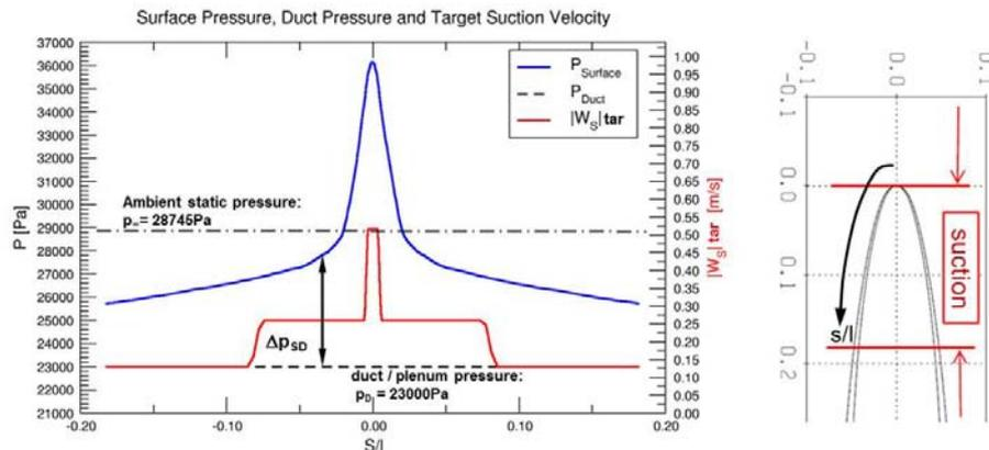
Figure 4: Surface pressure, duct pressure and target suction velocity vs. arc length along contour of cross section DV2
