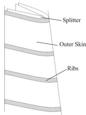
Figure 8: Modules of the novel leading edge design
