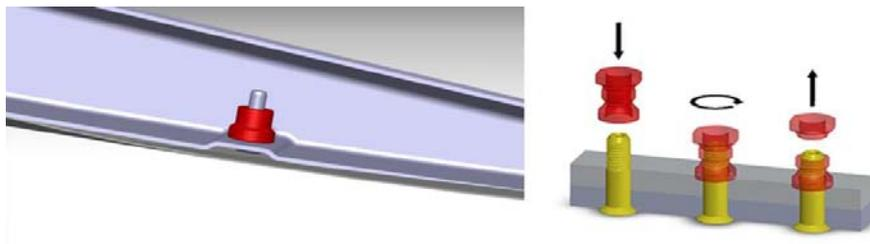
Figure 17: Demountable joining of outer skin with inner structure [5]
