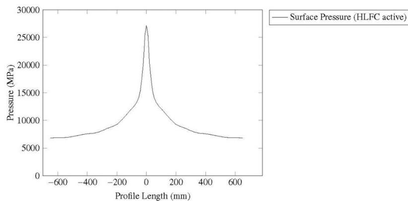
Figure 9: Pressure distribution for cruise condition and an active HLFC-System
