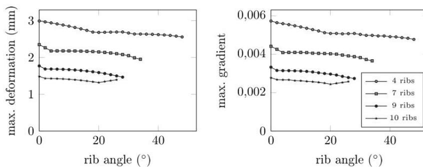
Figure 12: Maximum deformation and maximum angle for different rib configurations over the adjusted angle
