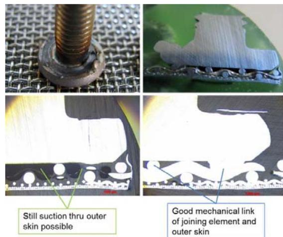
Figure 16: Laser joint cross section
