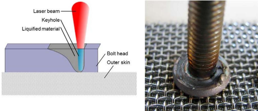
Figure 15: Joining process for outer skin
