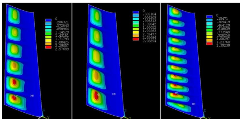
Figure 11: Maximum deflections for the configuration of 4, 5 and 10 ribs (left to right) at different angles
