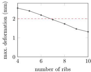
Figure 13: Maximum deformation over the number of ribs
