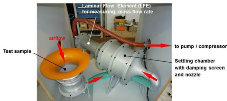
Figure 5: DLR Large Flow Meter (LFM) for measuring pressure loss characteristics of suction skins
