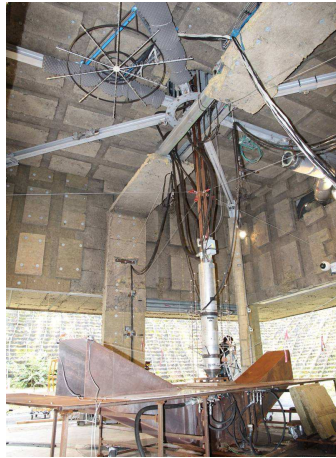
Figure 10: 115-microphone array set up in the Martel facility
