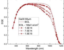
Figure 2 - EQE measurement on  $60\mu m$  Si heterojunction cell before and after irradiation with increasing 1MeV electron fluencies [2].
