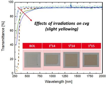
Figure 4 – Example of low cost coverglass optical degration with increasing 1MeV electrons fluence, and comparison with qualified coverglass.
