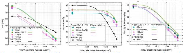
*Figure 3* - Variations of Voc, Jsc & Efficiency as measured in-house under AM1.5G spectrum at room temperature for p-type Gadoped Si heterojunction solar cells with various thicknesses. Comparison with commercial PERC cell.
