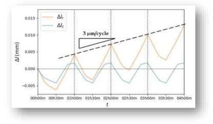
Figure 5 – Elongation of terrestrial standard interconnector ribbons with +/-140°C thermal cycles [14].
