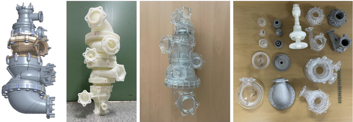
Figure 11: Single-shaft liquid methane and liquid oxygen turbopump for a 3tf class expander cycle rocket engine.
