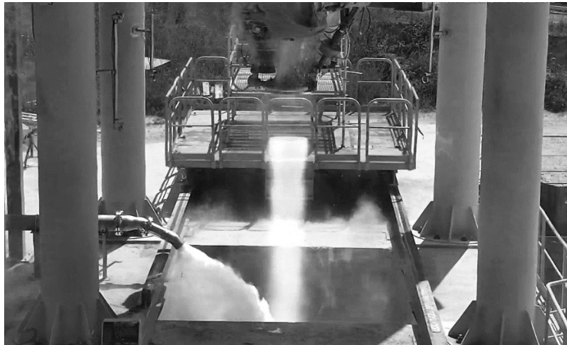
Figure 8: PROMETHEUS® Engine demonstrator during hot-firing tests
