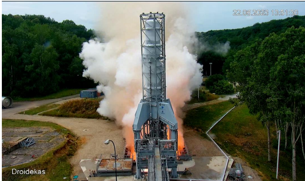
Figure 9: PROMETHEUS® Engine full ignition, ArianeGroup test center Vernon, France
