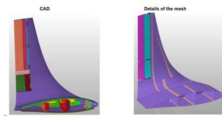
Figure 10: Model of the adaptive winglet
