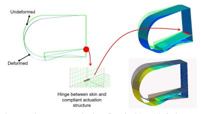
Figure 7: Using SAMCEF to develop a first (simple) model of a droop nose
