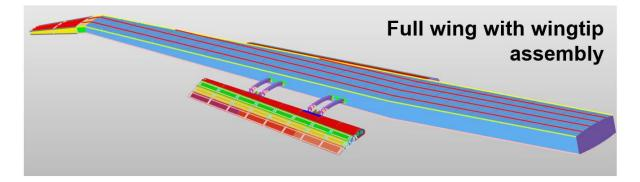
Figure 15: Wingtip mounted on the wing
