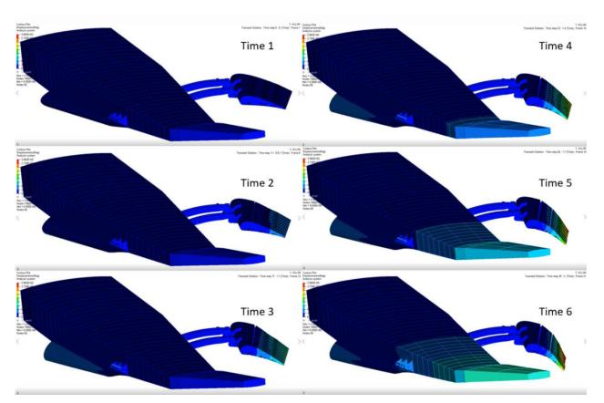
Figure 16: Motion and deformation of the full wing including the wingtip
