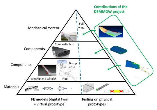
Figure 4: Pyramid approach to develop the model of the full morphing wing
