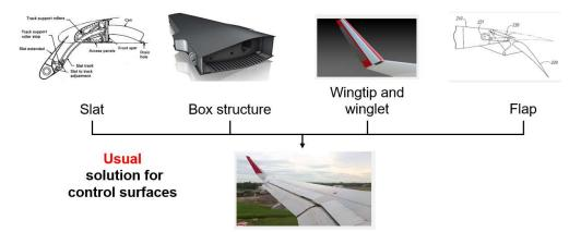
Figure 1: Illustration of a wing with classical high-lift devices, winglet and wingtip
