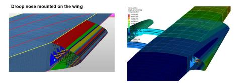
Figure 9: Droop nose mounted on the wing box
