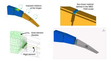
Figure 6: Using SAMCEF to develop a first (simple) model of an adaptive trailing edge component: definition of the hinges between the blocks
