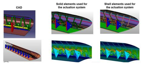
Figure 8: Model of the droop nose - comparison solid-shell
