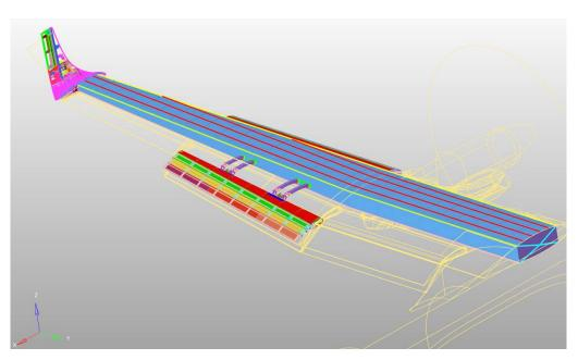
Figure 13: Global view of the full wing model with the winglet
