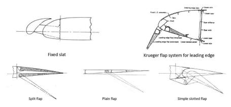
Figure 2: Conventional high lift devices for leading and trailing edges
