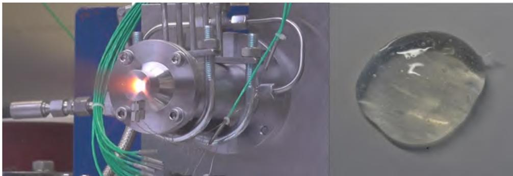
Figure 16: Left: Test firing of a nitromethane-based gelled monopropellant at the M11.4 test bench, Right: gelled monopropellant sample produced in the M3 laboratory
