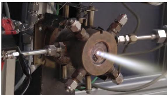
(a) Thruster operating with premixed HyNOx in a monopropellant-like system (see [46])
