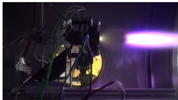
(b) Operation of thruster under vacuum conditions, burning a premixed  $N_2O/C_2H_6$  propellant [46]
