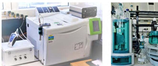
Figure 2: left: Gas chromatograph (Perkin Elmer); right: ion chromatograph (Metrohm)
