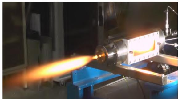
(b) Pressurized combustion chamber with optical access at M11.3
