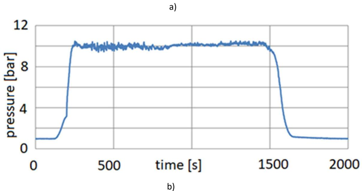
Fig.2. Typical pressure record inside detonative cone chamber for the case of stable CRD, a- part of pressure record by high frequency pressure sensor, b-pressure record by low frequency pressure sensor (average pressure in the chamber).
