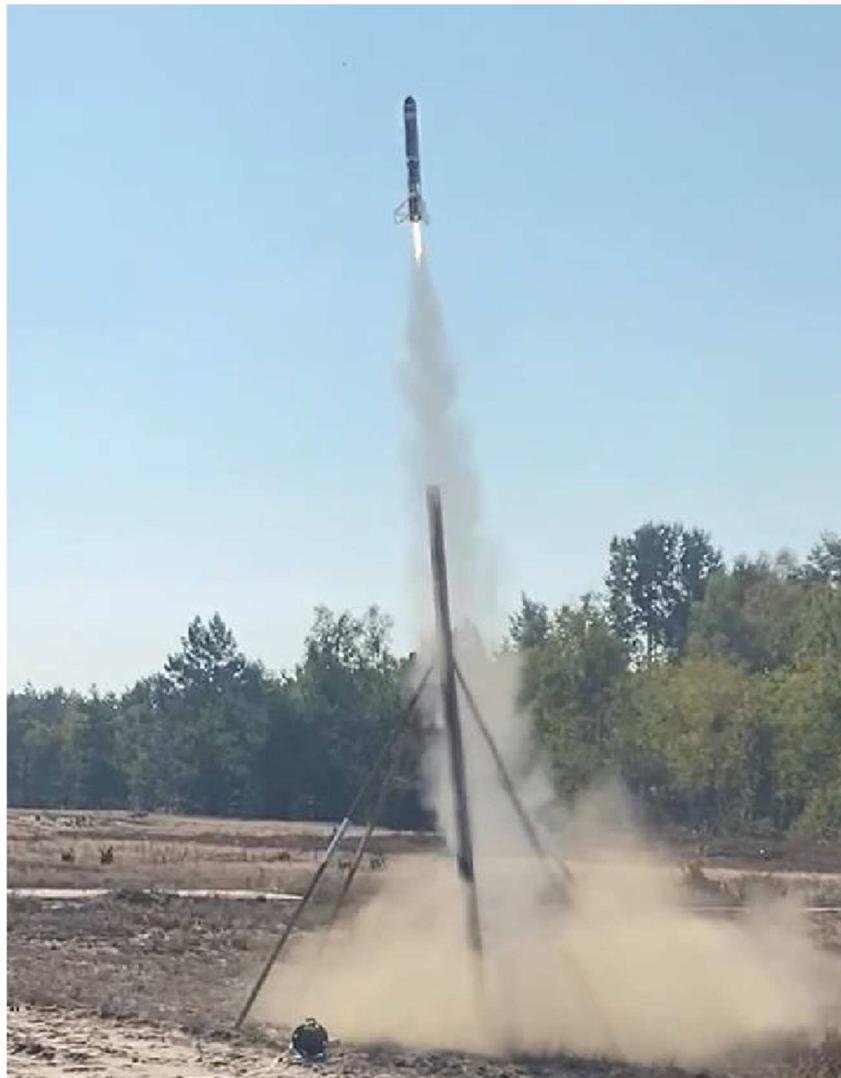
Fig.6. Picture of the launch of the first World's rocket powered by liquid propellants detonation engine.
