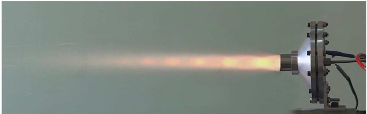
Fig.4. Test of the regenerative cooled cone detonation rocket engine supplied by liquid Nitrous Oxide and Liquid Propane.
