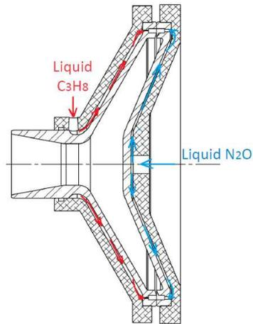
Fig.3. Schematic diagram of cone rocket engine with regenerative cooling system by both liquid propellants (please note that geometry of the engine are only approximate).
