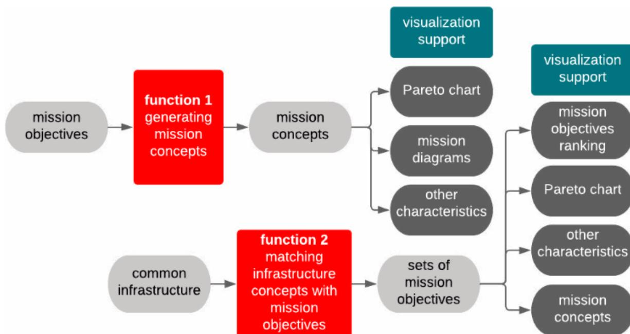
Figure 8 Connecting mission objectives to mission concepts and infrastructure design.
