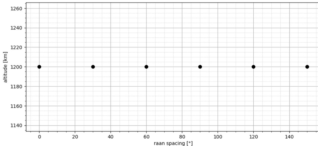
Figure 5 In this example, a fictional constellation with 6 planes and 10 satellites per plane is defined. All the satellites in a plane are deployed before the launcher manoeuvres to the next one with a RAAN drift, from  $0^\circ$  to  $30^\circ$  to  $60^\circ$  to  $90^\circ$  to  $120^\circ$  and to  $150^\circ$ .
