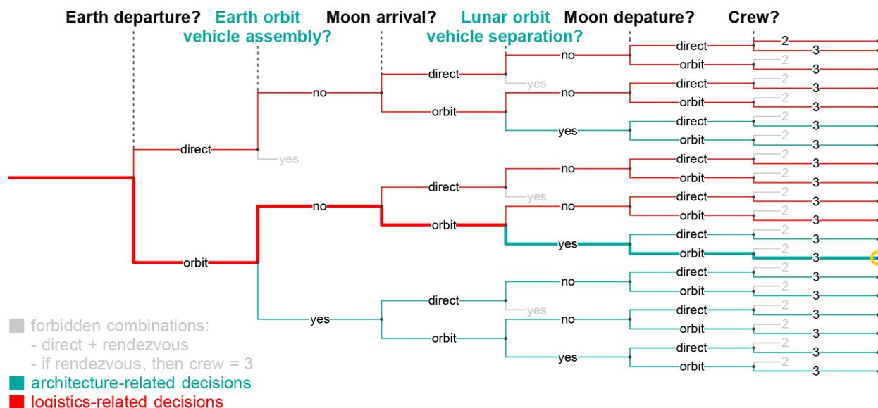
Figure 7 Decision tree for the design of the Apollo missions. This diagram is adapted from *System Architecture: Strategy and Product Development for Complex Systems* by Crawley, E., Cameron, B, and Selva, D. (2015) [19].
