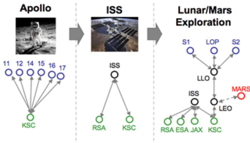
Figure 2 Space logistics paradigm evolution from “carry-along” (left), to “re-supply”, to more complex, mixed strategies with more nodes. Borrowed from [MIT Space Logistics project](#).
