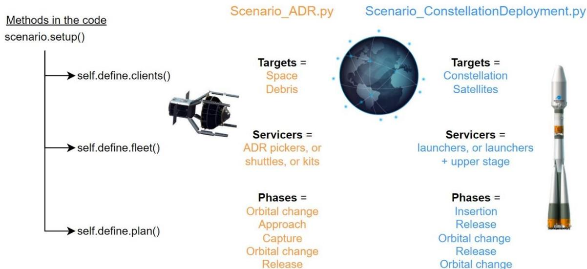
Figure 3 Sketch summarizing the setup() method in the code and the necessary elements for the simulation, for the ADR and constellation deployment scenarios. Three methods are called to define the clients, the fleet, and the plan (see section 2.3). The phases listed here in the plans are just examples [3].
