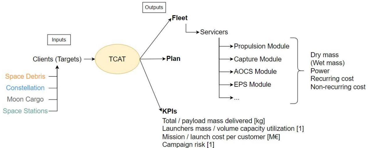
Figure 4 Description of the inputs and outputs of the tool [3].
