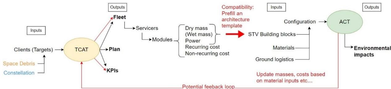
Figure 9 Highlight of the potential links (red arrows) foreseen to implement compatibility between TCAT and ACT.
