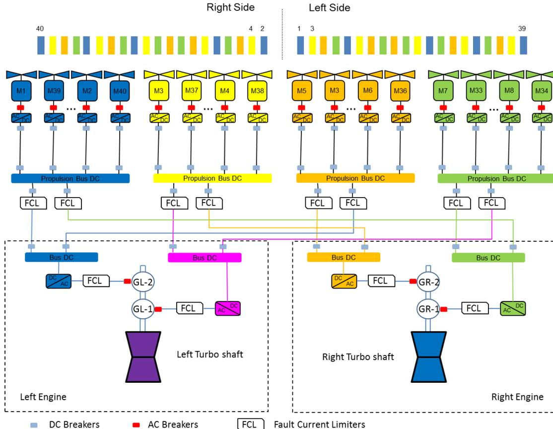
Figure 2: Electrical architecture set-up of the DRAGON configuration (example with 40 motors)
