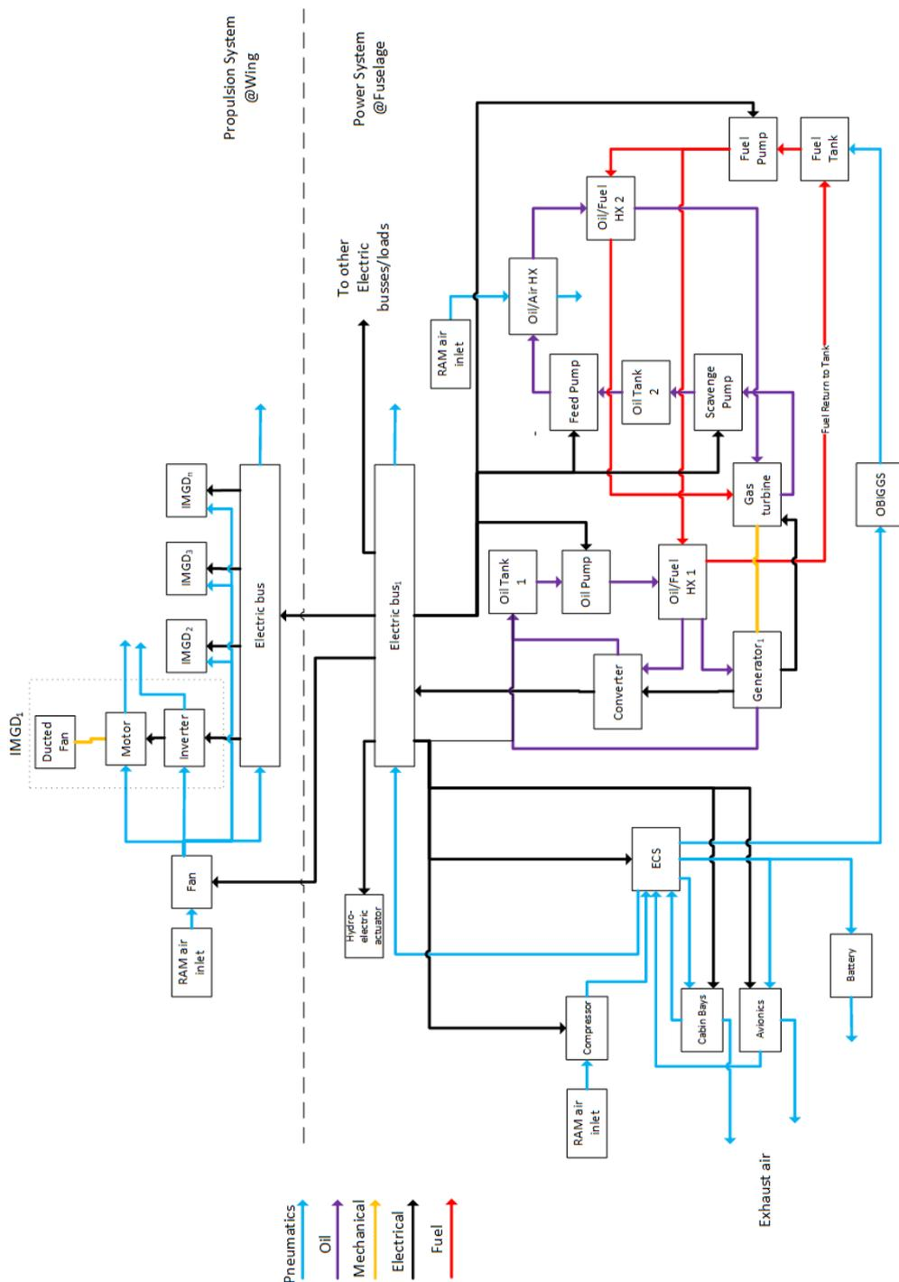
Figure 11: Schematic representation of interactions between pneumatic, hydraulic, mechanical, electrical and fuel systems for in-depth analysis of heat transfer.
