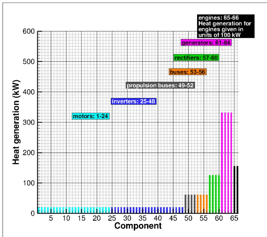
Figure 6: Heat losses in fully operational drive train components at ISA+18 temperature conditions for zero altitude and Mach number of 0.23.
