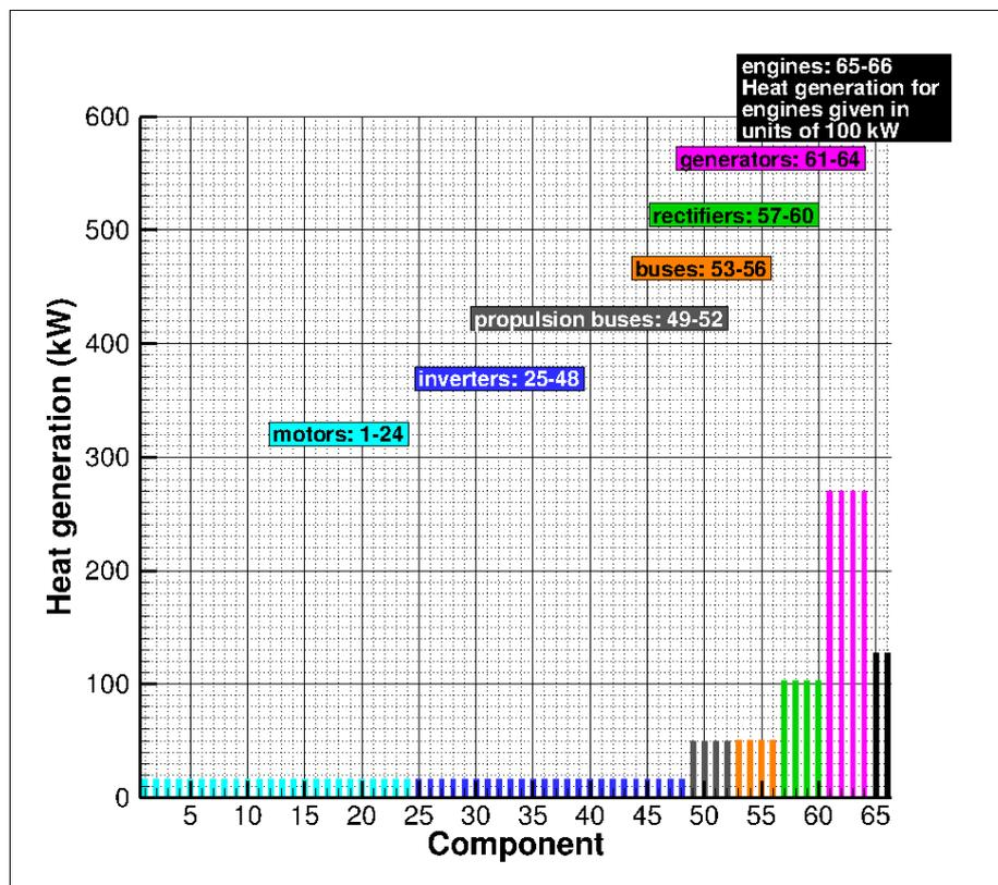
Figure 8: Heat losses in fully operational drive train components at ISA+18 temperature conditions for 11 km altitude and Mach number of 0.78.
