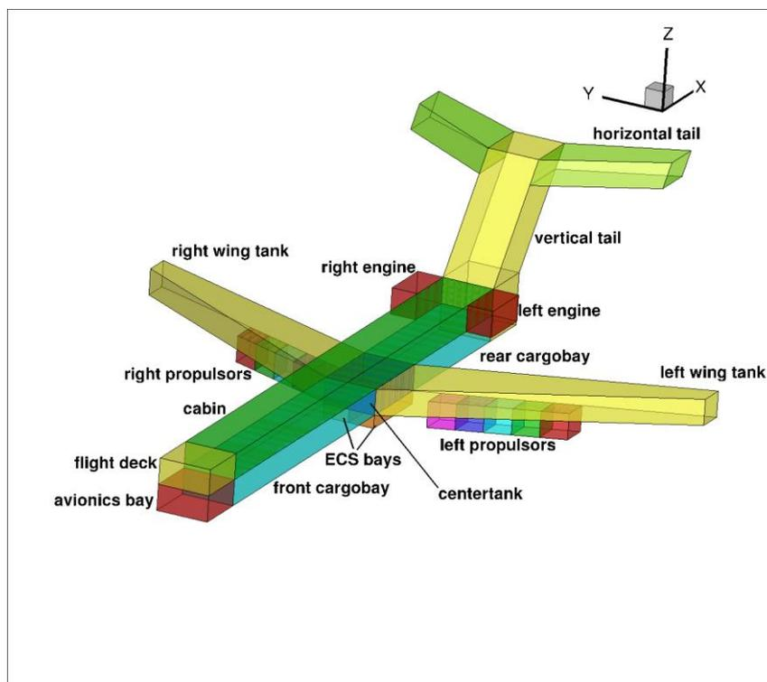
Figure 3: Conceptual representation of reduced thermal model (RTM) of SMR-con, based on main compartments.
