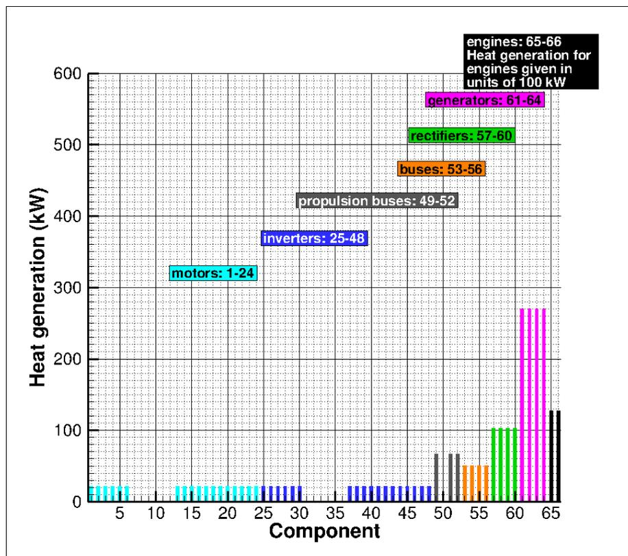
Figure 10: Heat losses in drive train components at ISA+18 temperature conditions for 11 km altitude and Mach number of 0.78; failure case in one of the propulsion buses.
