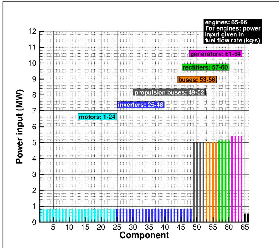
Figure 7: Power input to fully operational drive train components at ISA+18 temperature conditions for 11 km altitude and Mach number of 0.78.
