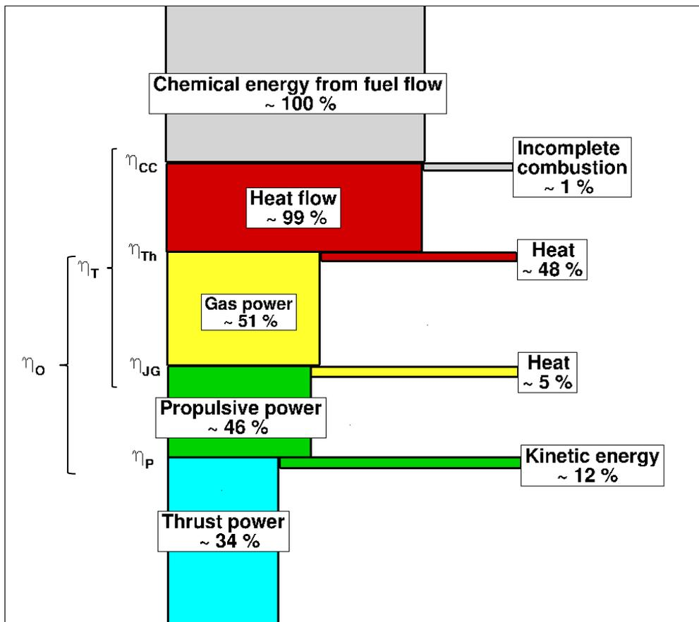
Figure 4: Schematic representation of powers, losses and efficiencies in an aircraft gas turbine engine (percentage numbers indicative only, based on 1980-technology status)
