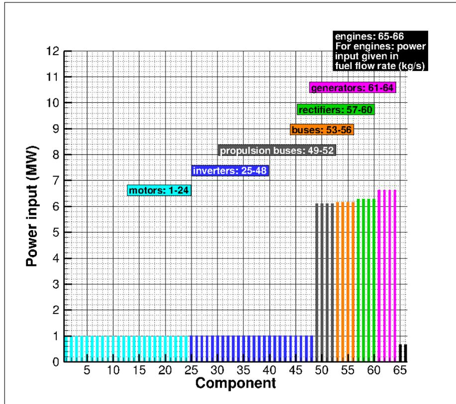
Figure 5: Power input to fully operational drive train components at ISA+18 temperature conditions for zero altitude and Mach number of 0.23.
