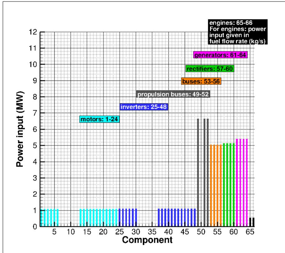
Figure 9: Power input to drive train components at ISA+18 temperature conditions for 11 km altitude and Mach number of 0.78; failure case in one of the propulsion buses.
