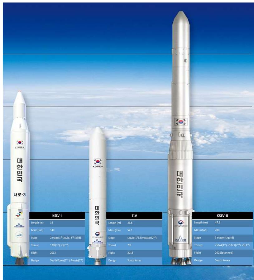
Figure 1: Configurations and specifications of the Korea Space Launch Vehicles developed by the KARI
