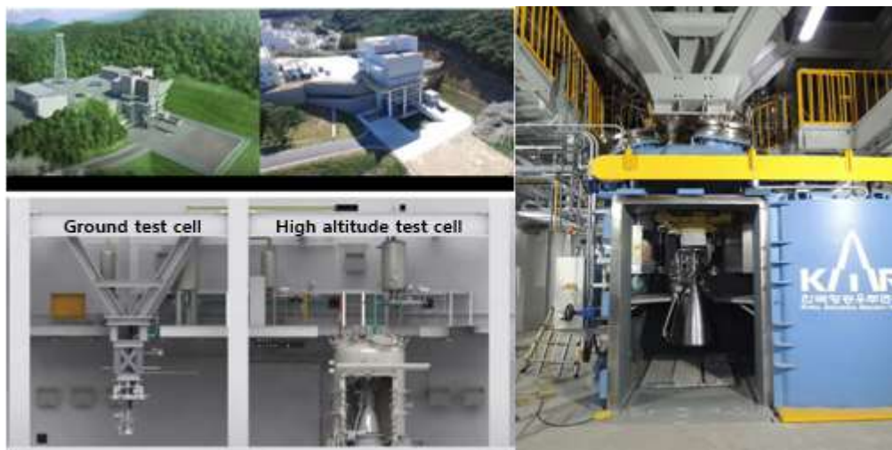
Figure 7: Upper-stage engine test facility [2, 10]
