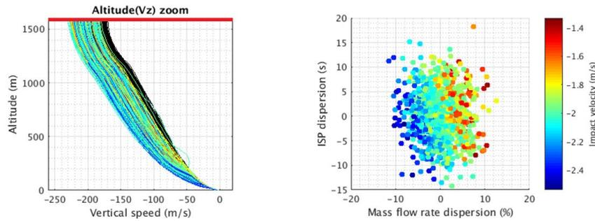
Figure 7. Monte-Carlo landing profiles and final conditions wrt propulsive dispersions
