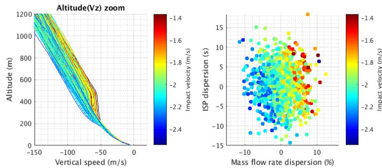
Figure 4. Impact of the terminal landing corridor
