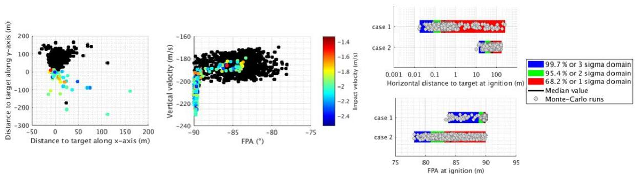
Figure 6. Monte-Carlo conditions at landing burn firing
