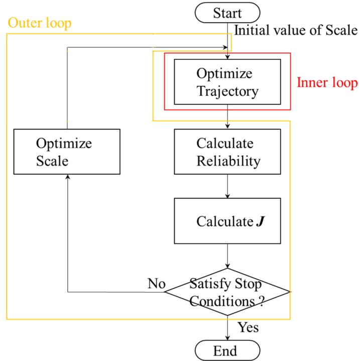
Figure 3.1: Concept design procedure
