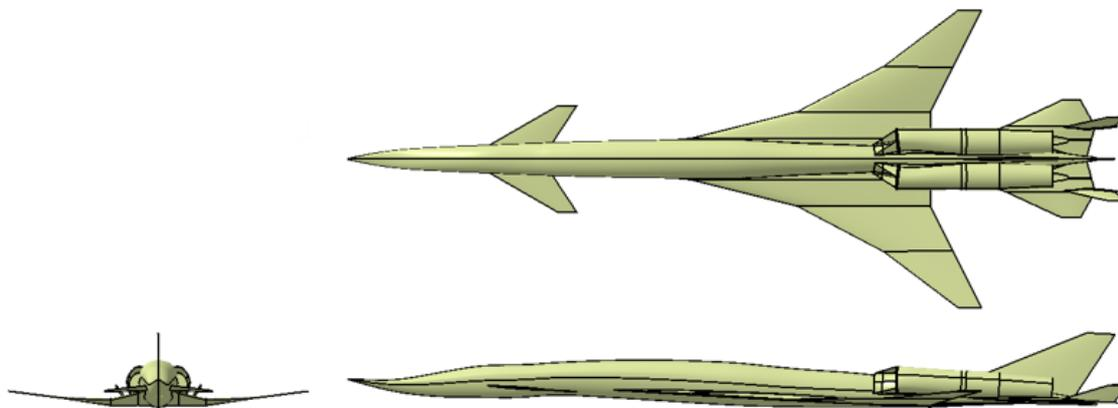
Figure 2.1: S4TD vehicle configuration
