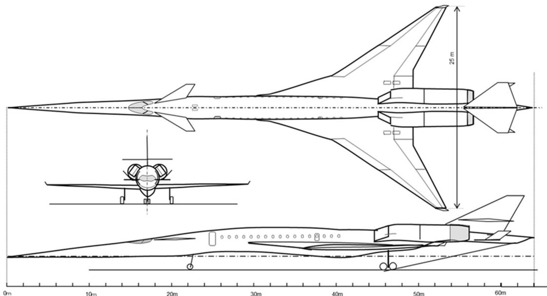
Figure 1: S4 technology reference aircraft
