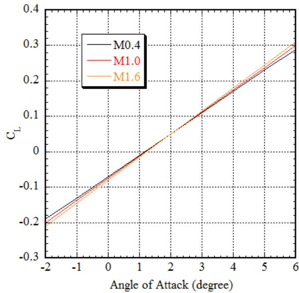
Figure 2.2(a): CL -  $\alpha$
